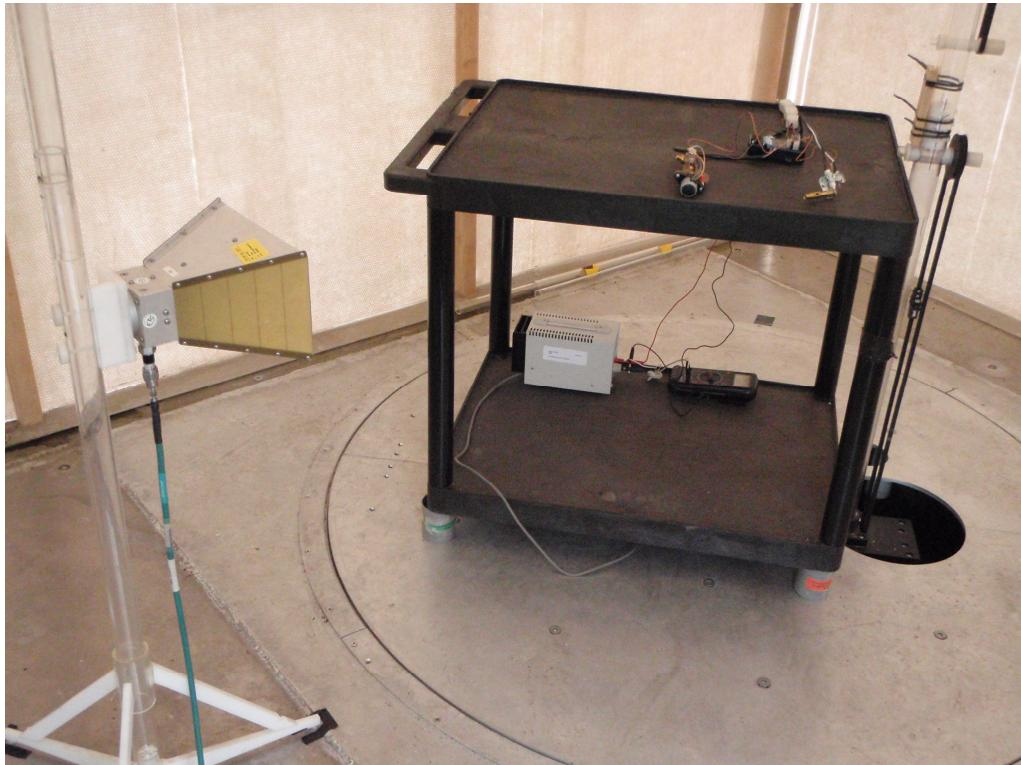
**Radiated Emissions Test Configuration 18GHz – 24GHz**
