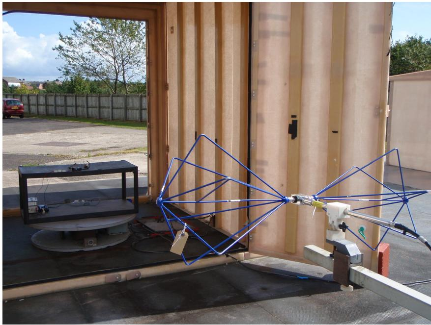
**Radiated Emissions Test Configuration 9kHz – 30MHz**
