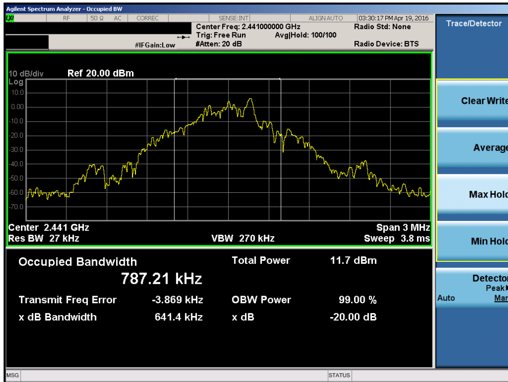
Plot 7-2. 20dB Bandwidth Plot (Bluetooth, 1Mbps – Ch. 39)
