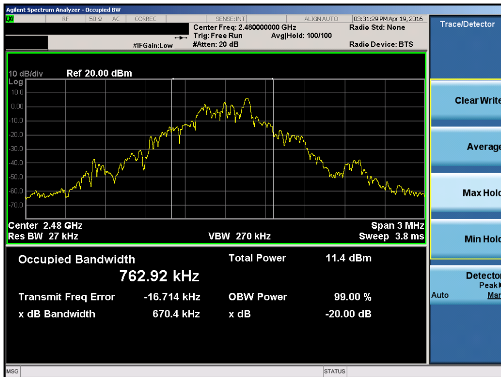
Plot 7-3. 20dB Bandwidth Plot (Bluetooth, 1Mbps – Ch. 78)
