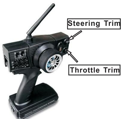
Throttle Trim is used to slightly trim the throttle servo When the trigger is at Neutral position.
