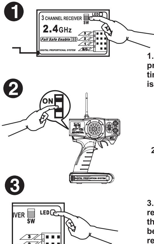
1. Turn on the receiver power, press SW switch, at the same time, the receiver's red LED is flashing.
