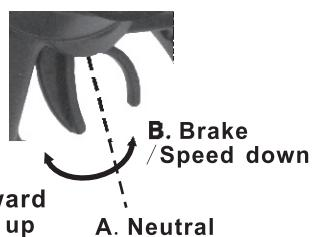
1. Push the trigger forwards to allow the vehicle to speed down or brake.
