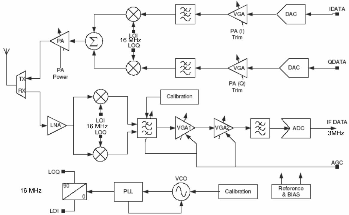
The radio comprises a low-IF receive path and a direct up-conversion transmit path, which converge at the TX/RX switch. This switch includes the necessary matching components such that a  $200\Omega$  differential antenna may be directly connected without external components. Alternatively, a balun can be used for single ended antennas.
