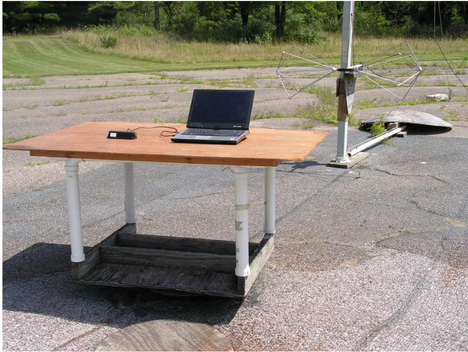
Photograph 6.7. Digital Emissions Test Setup on OATS
