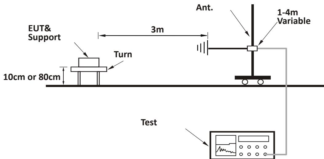
**TEST REPORT****For Radiated emission 1GHz to 40GHz:**
