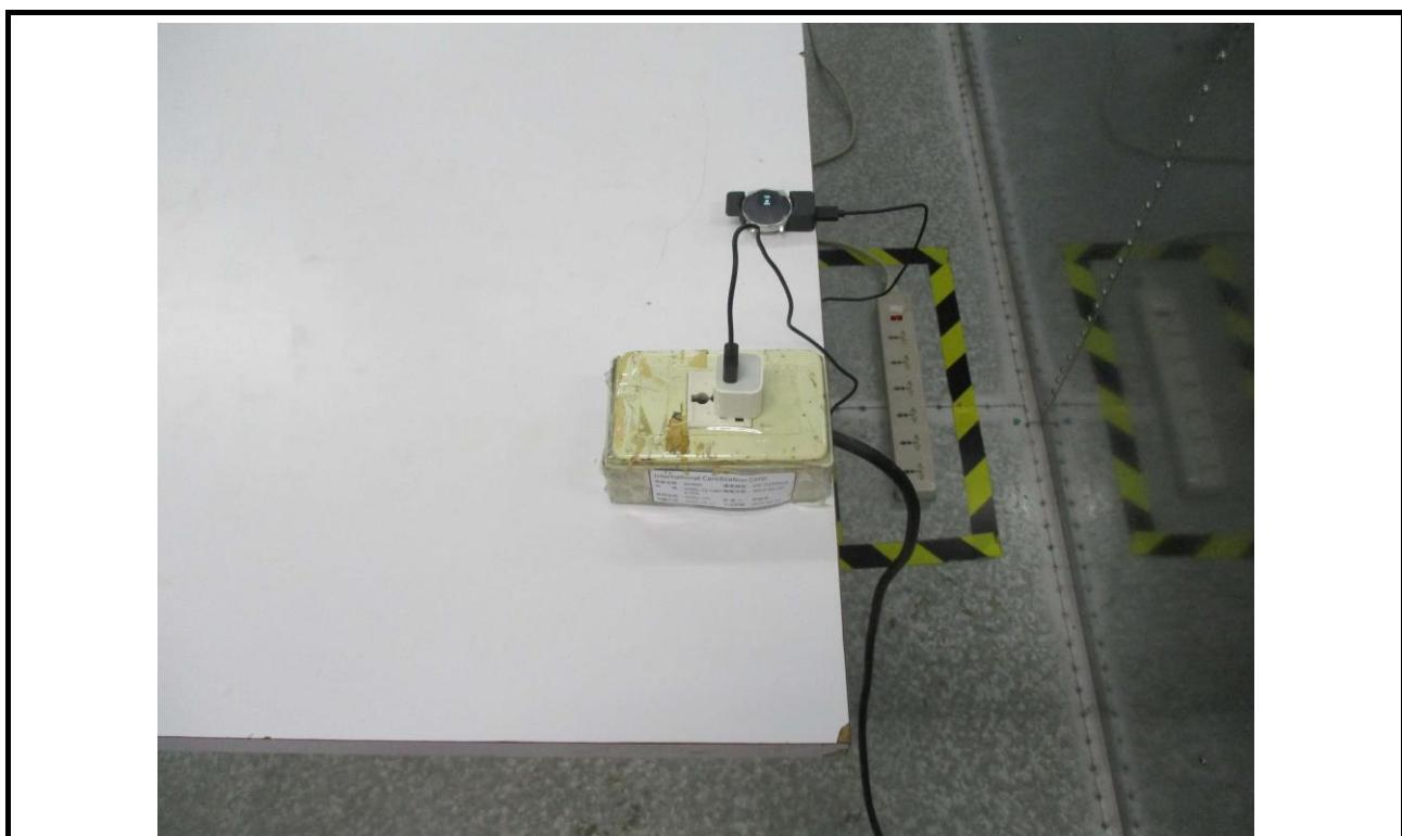
**Radiated Emission Below 1GHz Test (Battery Mode)**
