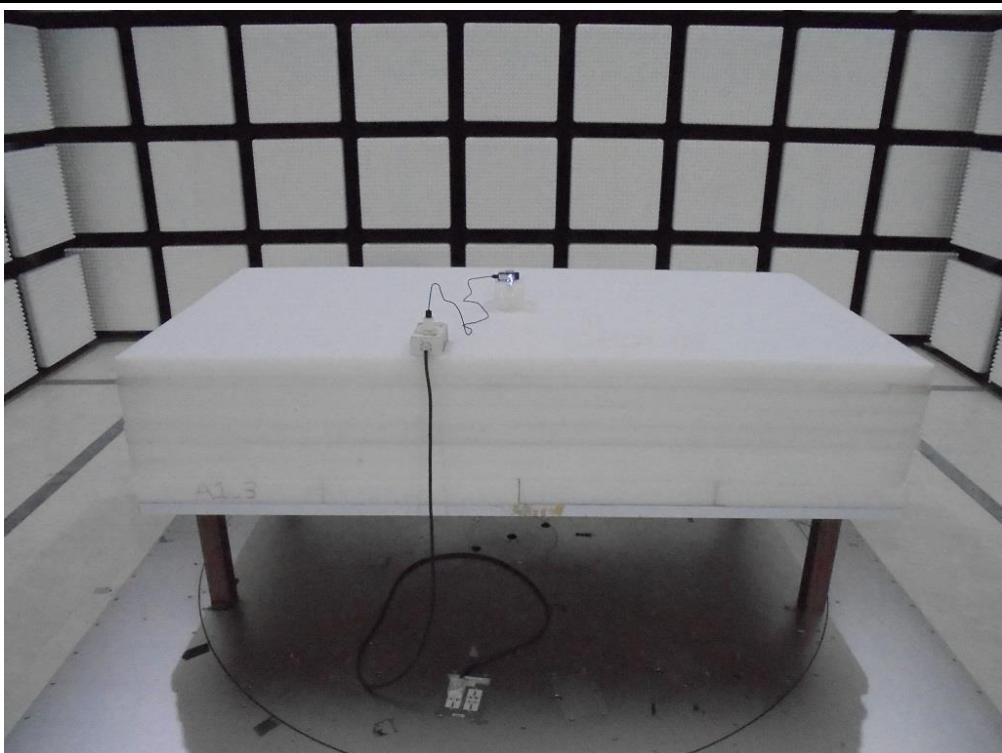
**Radiated Emission Below 1GHz Test (Charging Mode)**
