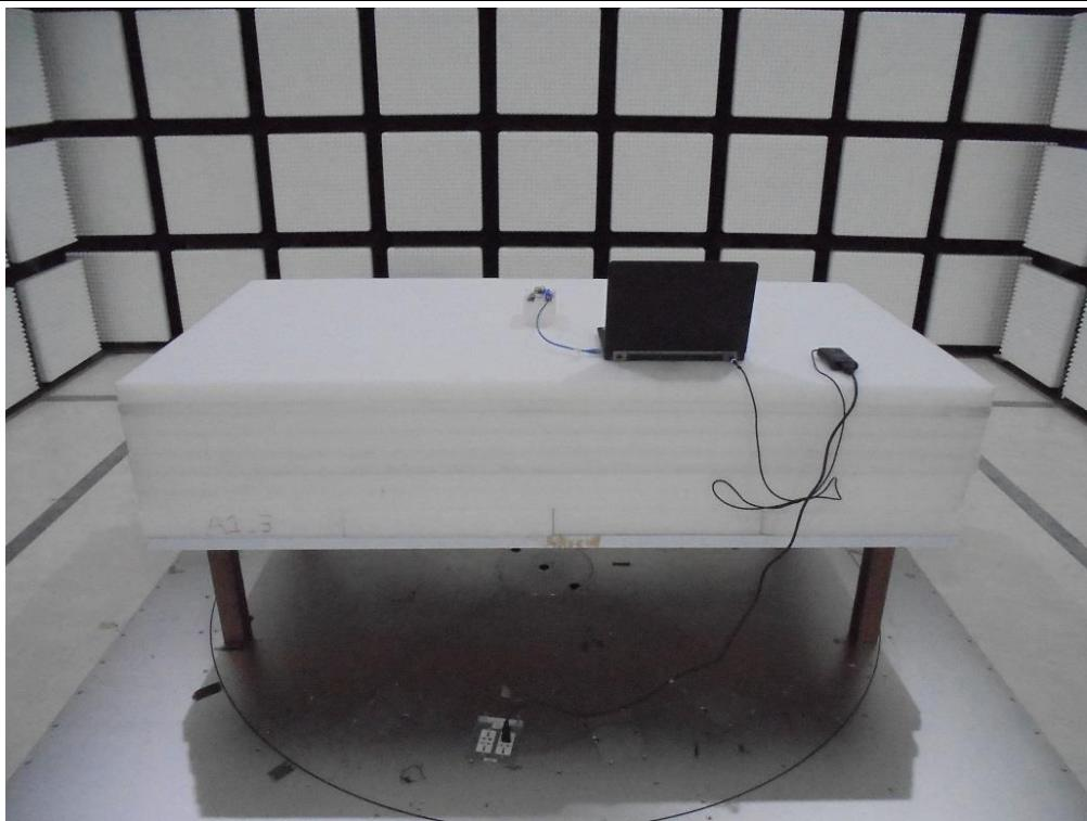
**Radiated Emission Below 1GHz Test (Battery Mode)**
