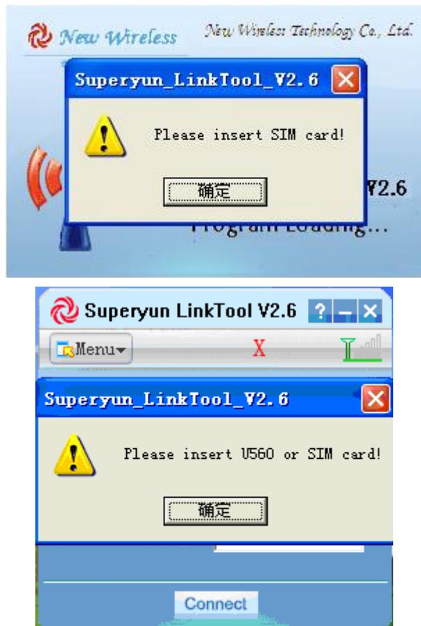
If Linktool pop up this windows when start-up, start search or connect, then check if the SIM card is inserting device, if do , get it out and plug in again
