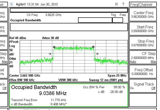
**10MHz EBW, High Channel 16QAM**
