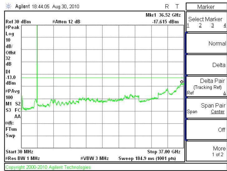
**5 MHZ 64QAM CONDUCTED SPURIOUS, MID CHANNEL, P=35 dBm**
