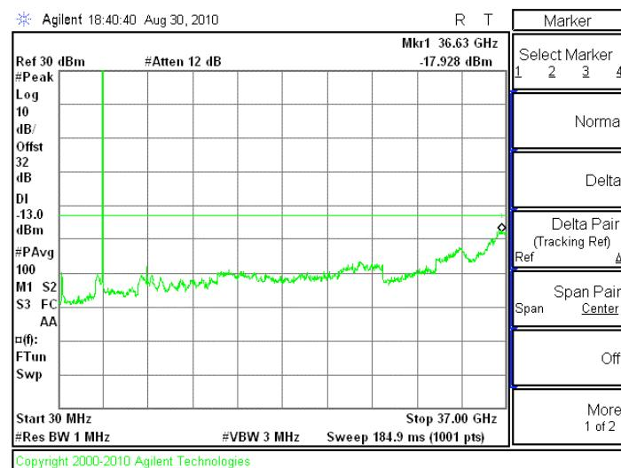
**5 MHZ 64QAM CONDUCTED SPURIOUS, 3652.5 MHzLOW CHANNEL, P=27 dBm**
