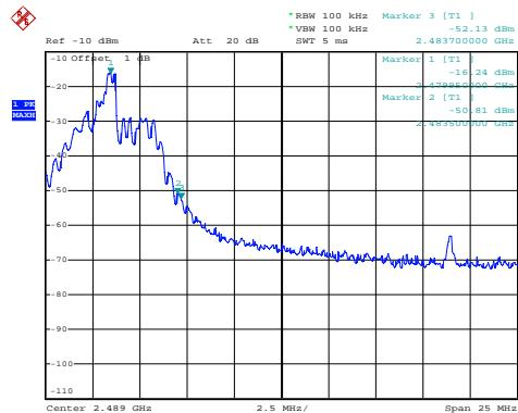
Figure 6. Plot of the Surious Emission(Conducted)
