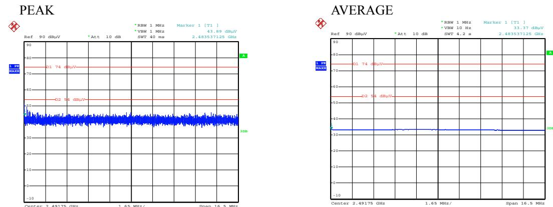
Figure 5. Plot of the Bandedge Compliance(Conducted)
