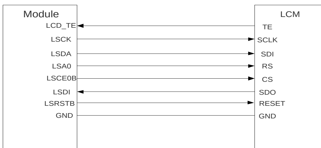
Figure 20: Reference Circuit Design for LCM Interface
