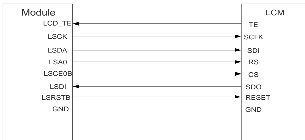
Figure 20: Reference Circuit Design for LCM Interface
