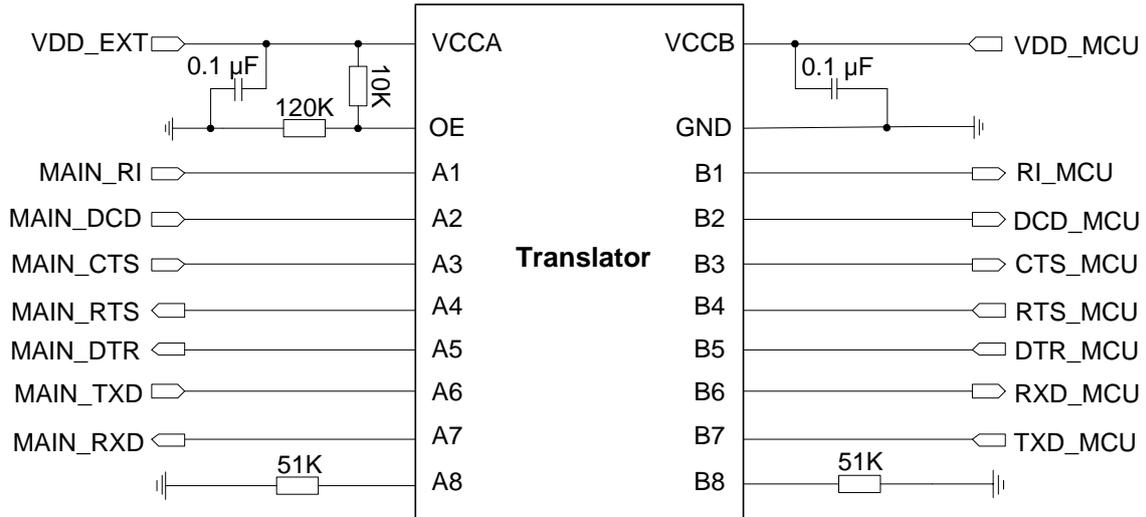
**Figure 23: Reference Design of UART with Level-shifting Chip**
