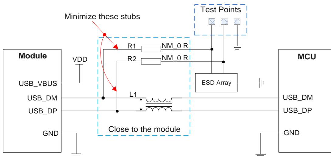
**Figure 17: Reference Design of USB 2.0 Interface**
