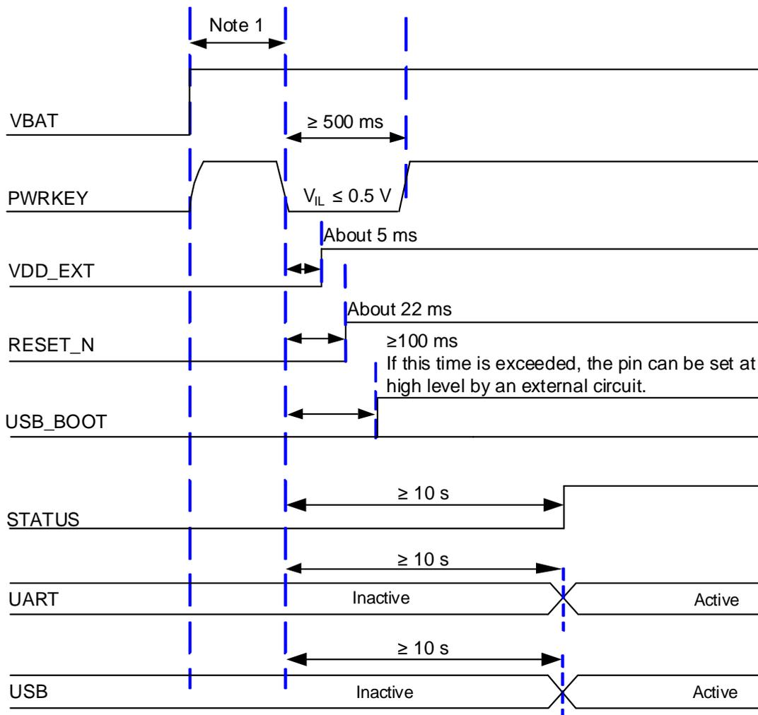
Figure 12: Power-up Timing
