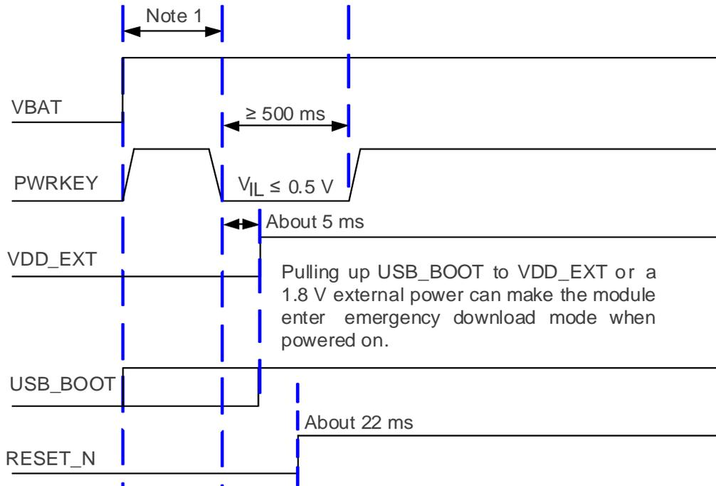
Figure 19: Timing Sequence for Entering Emergency Download Mode
