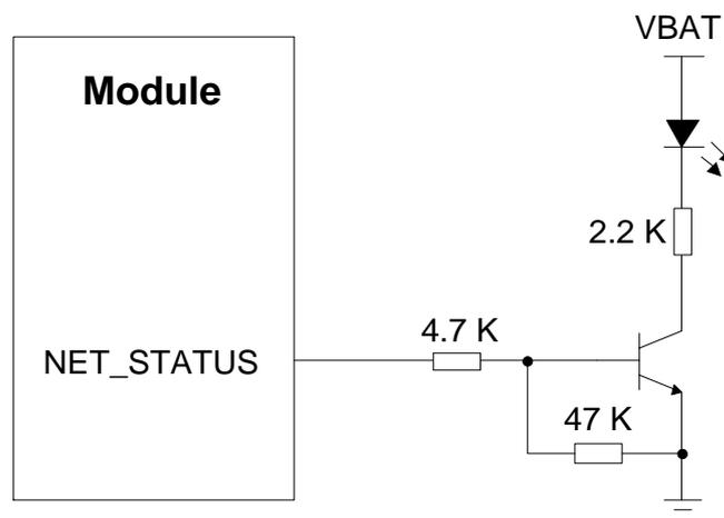
**Figure 27: Reference Design of Network Status Indication**
