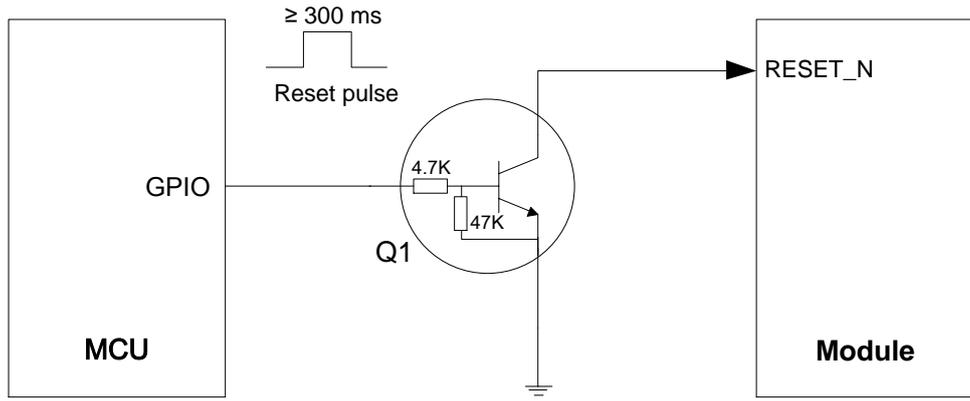
Figure 14: Reference Circuit of RESET\_N with Driving Circuit
