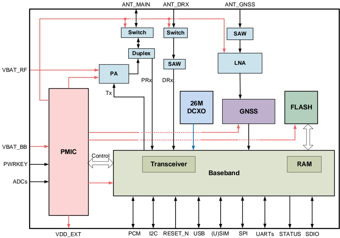
**Figure 1: Functional Diagram**
