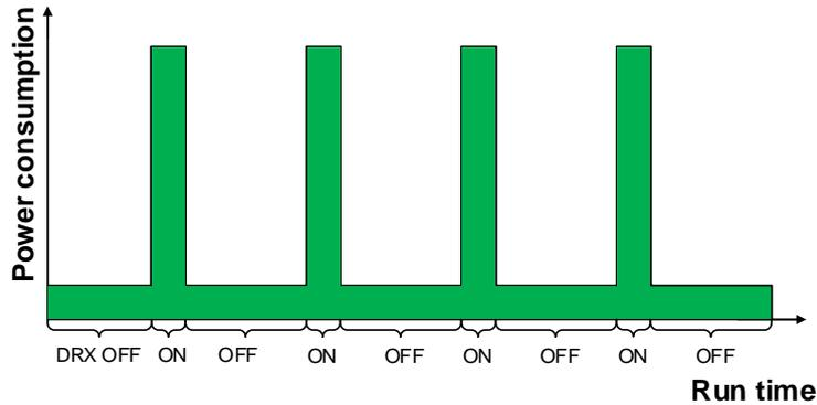
**Figure 3: Module Power Consumption in Sleep Mode**
