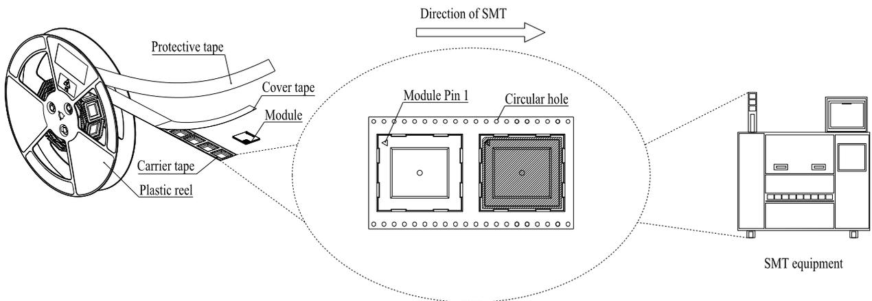
**Figure 44: Mounting Direction**
