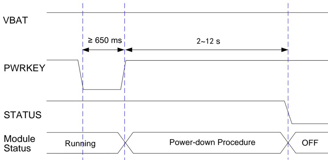
**Figure 13: Power-down Timing**
