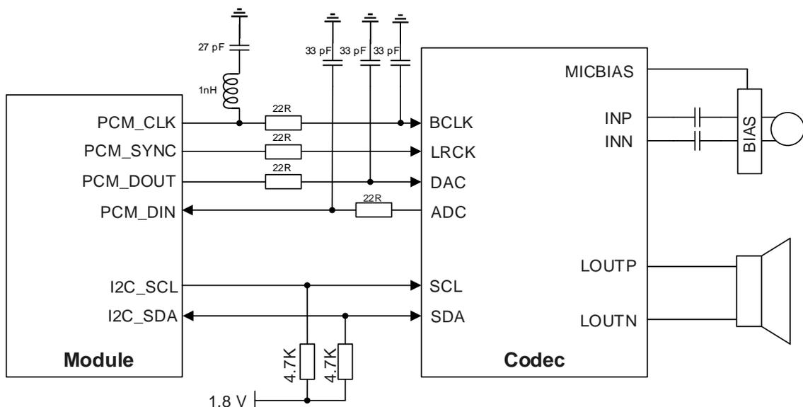
**Figure 26: Reference Design of PCM and I2C Interfaces**
