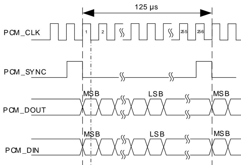
**Figure 25: Timing Sequence for Short Frame Mode**
