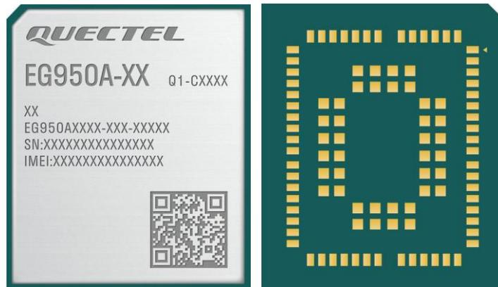
Figure 40: Top & Bottom Views of the Module
