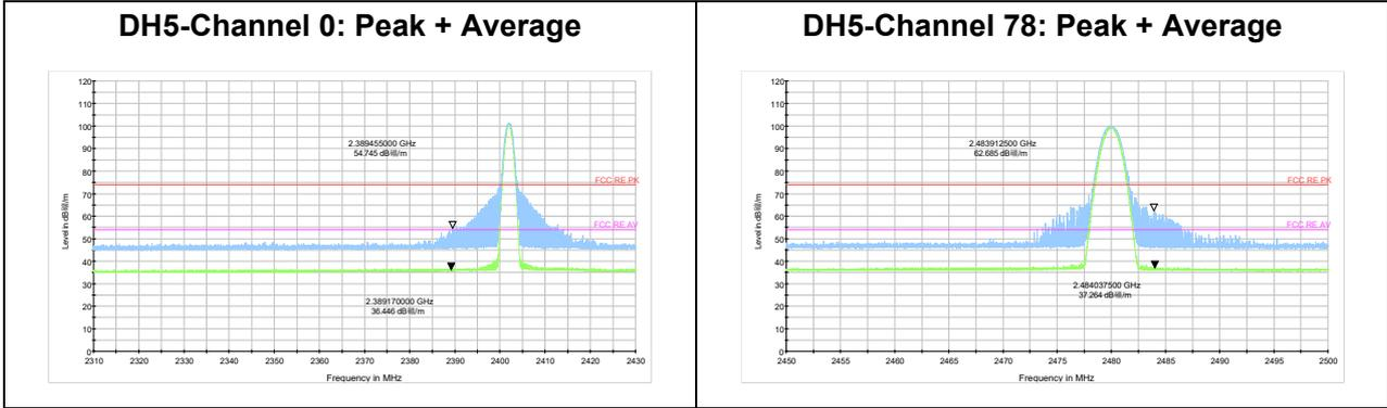
The bandage was performed in all EDR mode (2DH5 and 3DH5), 3DH5 was selected as the worse condition. The test data of the worst-case condition was recorded in this report.
