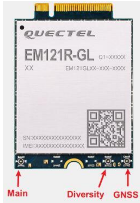
Figure 33: Antenna Connectors on the EM121R-GL Module
