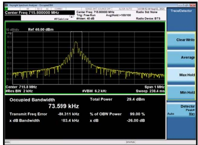
NB-IoT Band 12 QPSK 15KHz 12@0 CH-Low
