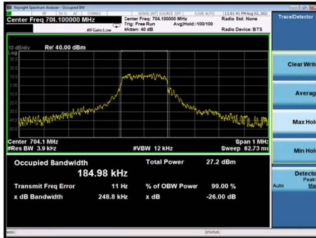
NB-IoT Band 17 QPSK 15KHz 12@0 CH-Middle
