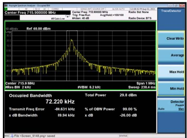
NB-IoT Band 17 QPSK 3.75KHz 1@0 CH-Low
