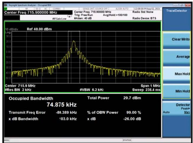
NB-IoT Band 17 QPSK 15KHz 12@0 CH-Low
