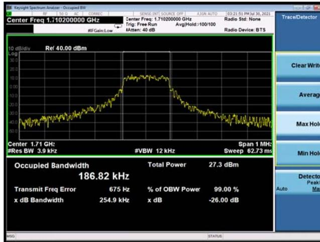
NB-IoT Band 4 QPSK 15KHz 12@0 CH-Middle
