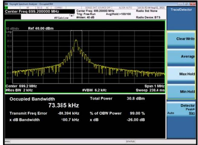
NB-IoT Band 12 QPSK 3.75KHz 1@0 CH-Middle
