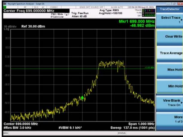
NB-IoT Band 12 QPSK 15KHz 12@0 CH- High
