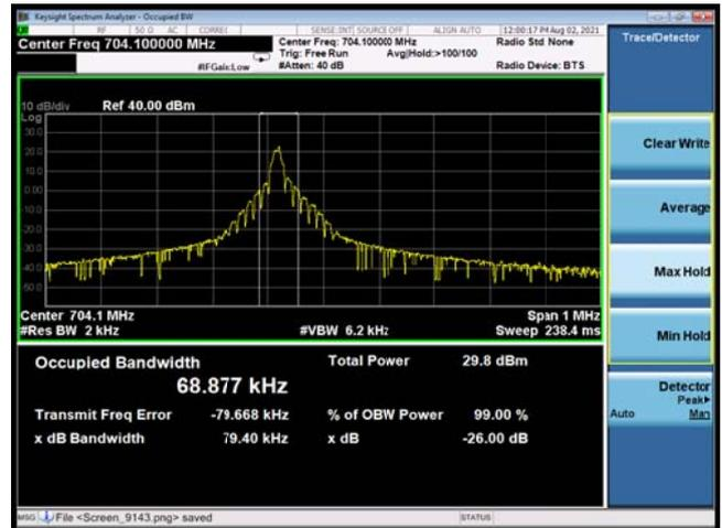
NB-IoT Band 17 BPSK 3.75KHz 1@0 CH-Middle
