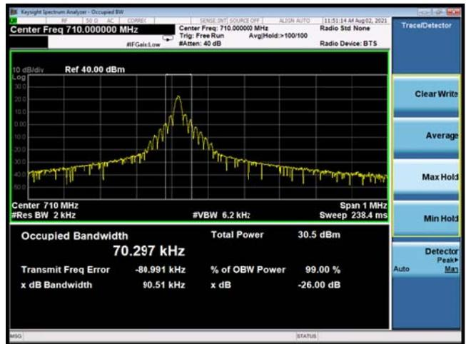
NB-IoT Band 17 QPSK 3.75KHz 1@0 CH-High
