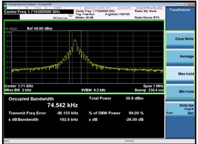
NB-IoT Band 4 QPSK 3.75KHz 1@0 CH-Middle
