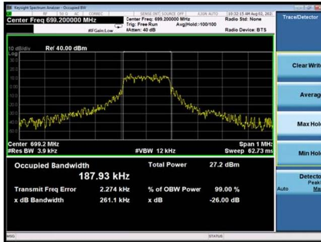
NB-IoT Band 12 QPSK 15KHz 12@0 CH-Middle
