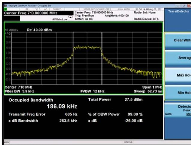
NB-IoT Band 17 QPSK 15KHz 12@0 CH-High
