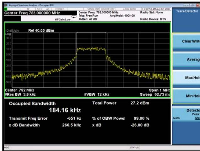
NB-IoT Band 13 QPSK 15KHz 12@0 CH-High
