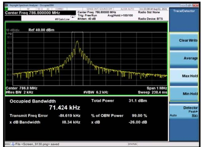
NB-IoT Band 13 QPSK 15KHz 12@0 CH-Low
