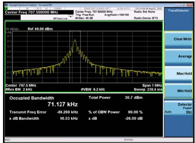
NB-IoT Band 12 QPSK 3.75KHz 1@0 CH-High
