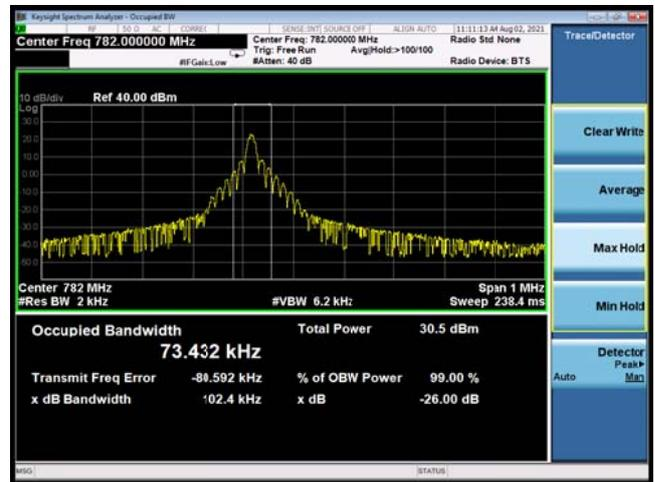
NB-IoT Band 13 QPSK 3.75KHz 1@0 CH-High
