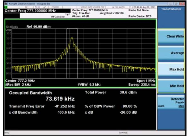
NB-IoT Band 13 QPSK 3.75KHz 1@0 CH-Middle
