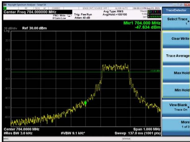
NB-IoT Band 17 QPSK 15KHz 12@0 CH- High
