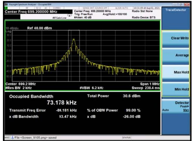
NB-IoT Band 12 BPSK 3.75KHz 1@0 CH-Middle
