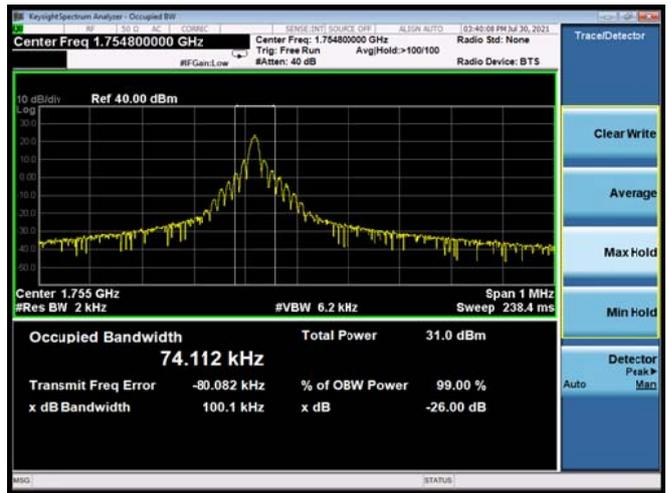
NB-IoT Band 4 QPSK 15KHz 12@0 CH-Low
