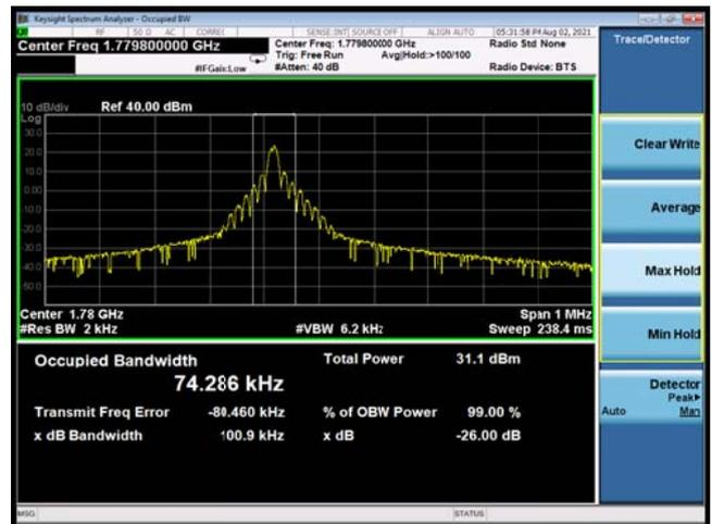
NB-IoT Band 66 QPSK 15KHz 12@0 CH-Low
