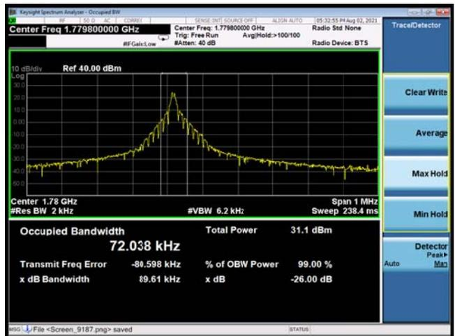
NB-IoT Band 66 QPSK 3.75KHz 1@0 CH-Low
