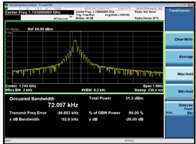
NB-IoT Band 66 QPSK 3.75KHz 1@0 CH-High
