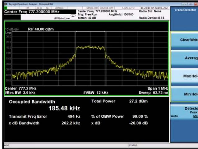
NB-IoT Band 13 QPSK 15KHz 12@0 CH-Middle
