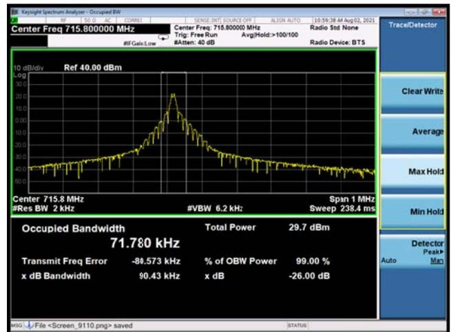
NB-IoT Band 12 QPSK 3.75KHz 1@0 CH-Low
