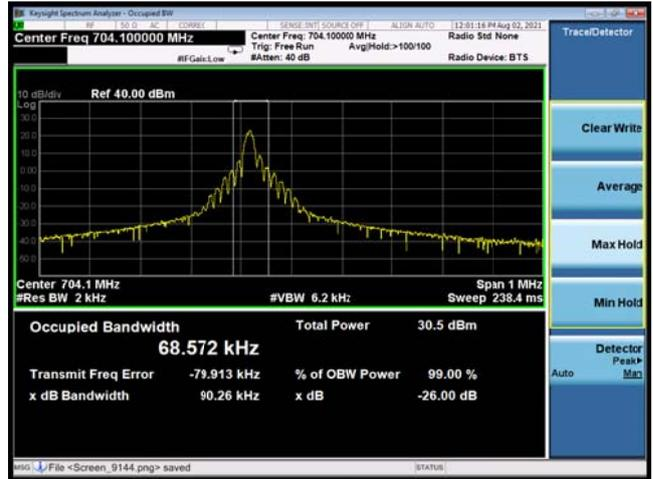
NB-IoT Band 17 QPSK 3.75KHz 1@0 CH-Middle
