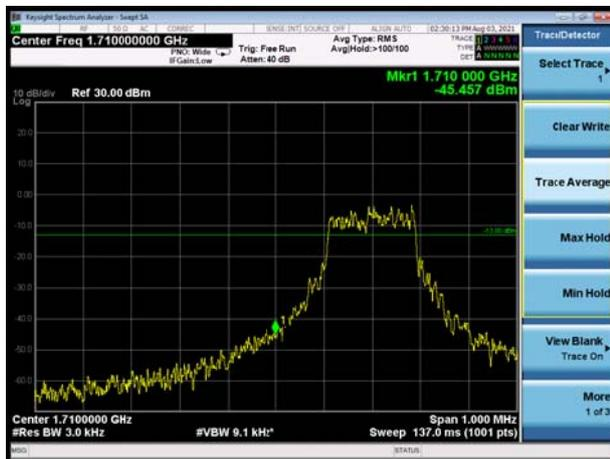
NB-IoT Band 4 QPSK 15KHz 12@0 CH- High
