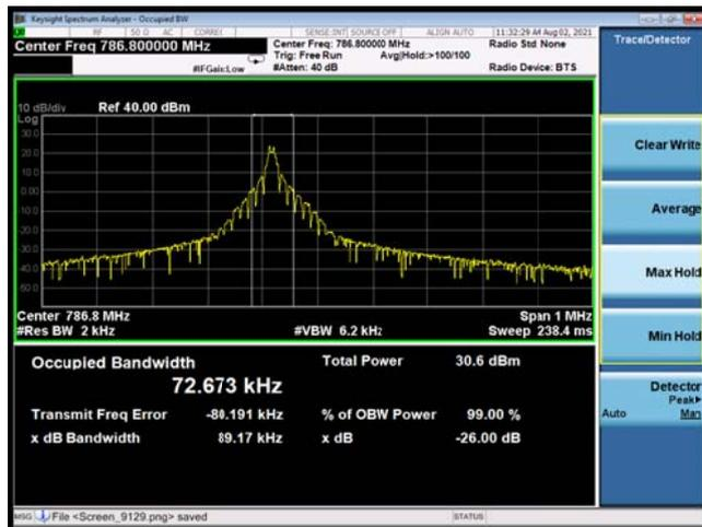
NB-IoT Band 13 QPSK 3.75KHz 1@0 CH-Low
