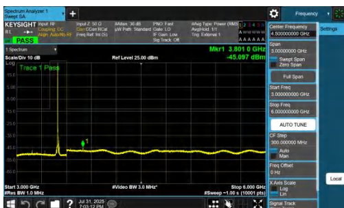
NTNV-DC_7A_n77A-PC2-30-5+15-M+M-QPSK-IDLE-DFT-QPSK-I nner 1RB Left-3000-6000-PASS
