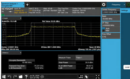
NTNV-n77(3450-3550)-PC2-30-20-M-CP-64QAM-Outet_Full-Ant1-PA
