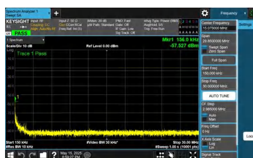
NTNV-n71-PC3-15-5-H-DFT-BPSK-Inner 1RB Right-0.15-30-PASS
