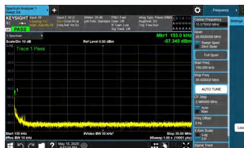
NTNV-n71-PC3-15-5-H-DFT-BPSK-Inner 1RB Left-0.15-30-PASS
