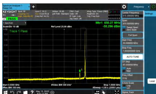
NTNV-n71-PC3-15-5-H-DFT-BPSK-Inner 1RB Left-30-1000-PASS
