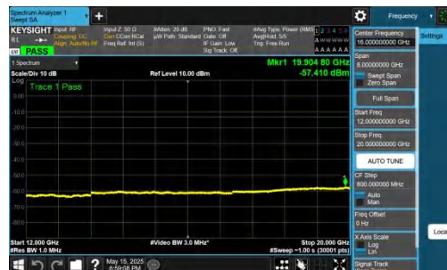
NTNV-n12-PC3-15-5-L-DFT-BPSK-Inner 1RB Left-12000-20000-PAS
