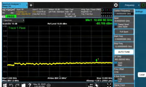
NTNV-n12-PC3-15-5-L-DFT-BPSK-Inner 1RB Left-3000-12000-PAS
