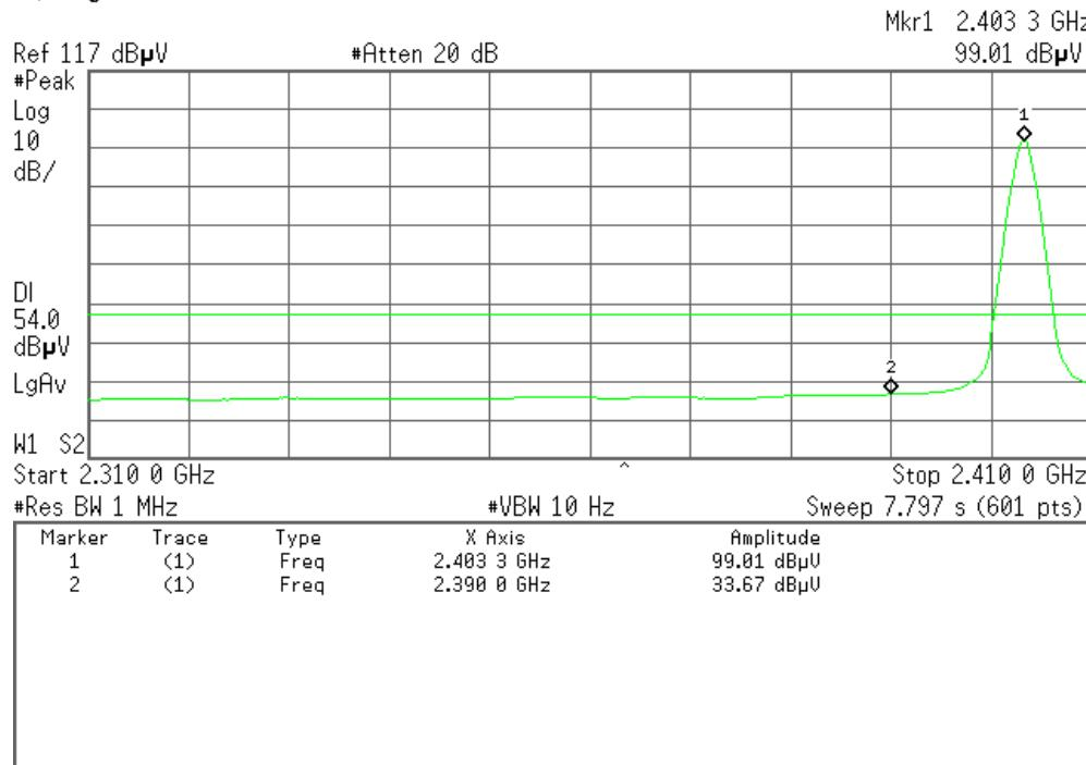
**Band Edges (CH-High)****Detector mode: Peak****Polarity: Vertical**
