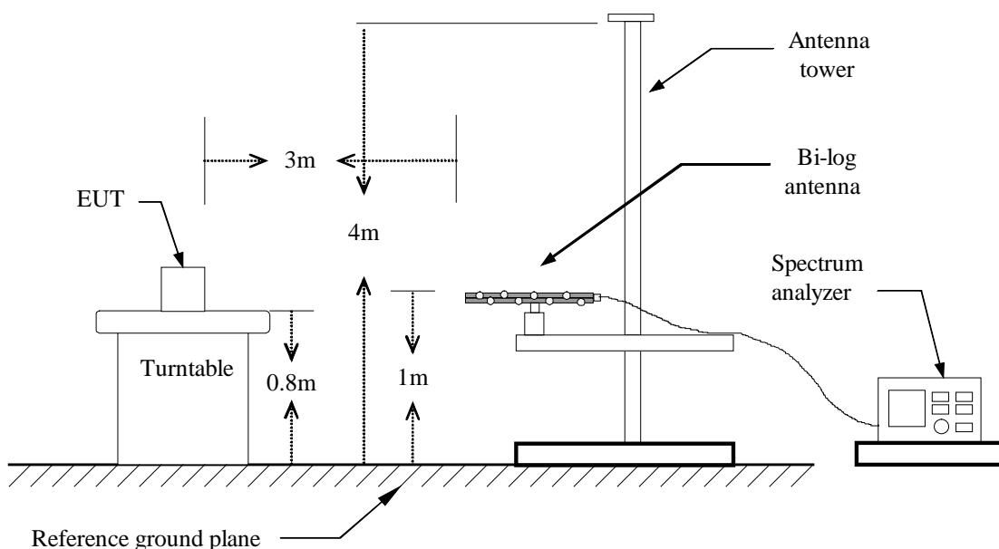
**Above 1 GHz**
