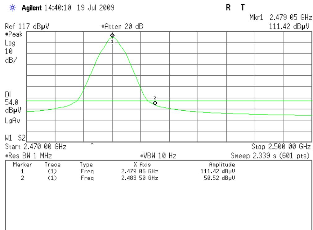
**Detector mode: Peak****Polarity: Horizontal**
