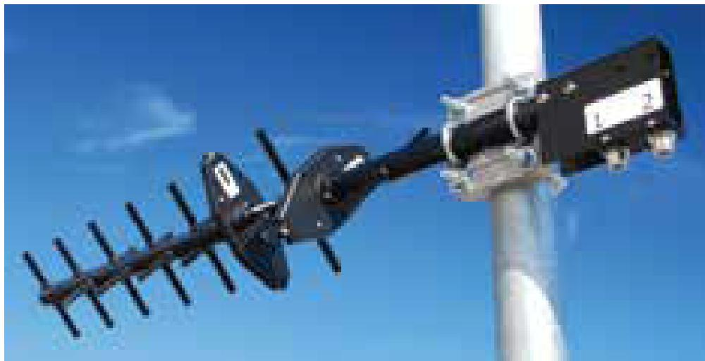
The 700 MHz MiMO Yagi Antenna with Dual Polarization is a high gain, premium quality antenna with excellent port to port isolation. Manufactured using high strength 6061-T6 aluminum, they will withstand heavy ice, high wind and other harsh conditions. The entire antenna is anodized for aesthetic appearance and corrosion resistance.
