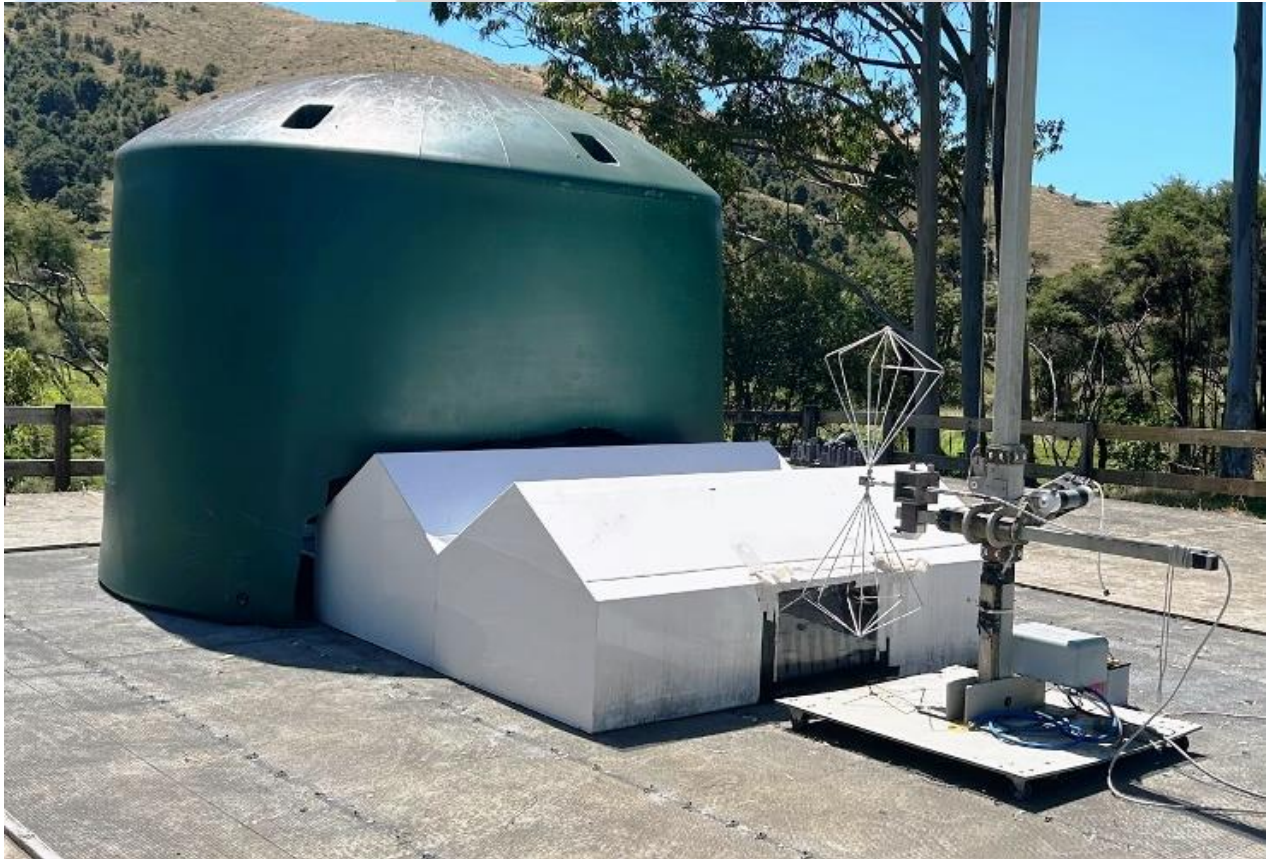
Biconical Antenna pointing towards Test Enclosure
