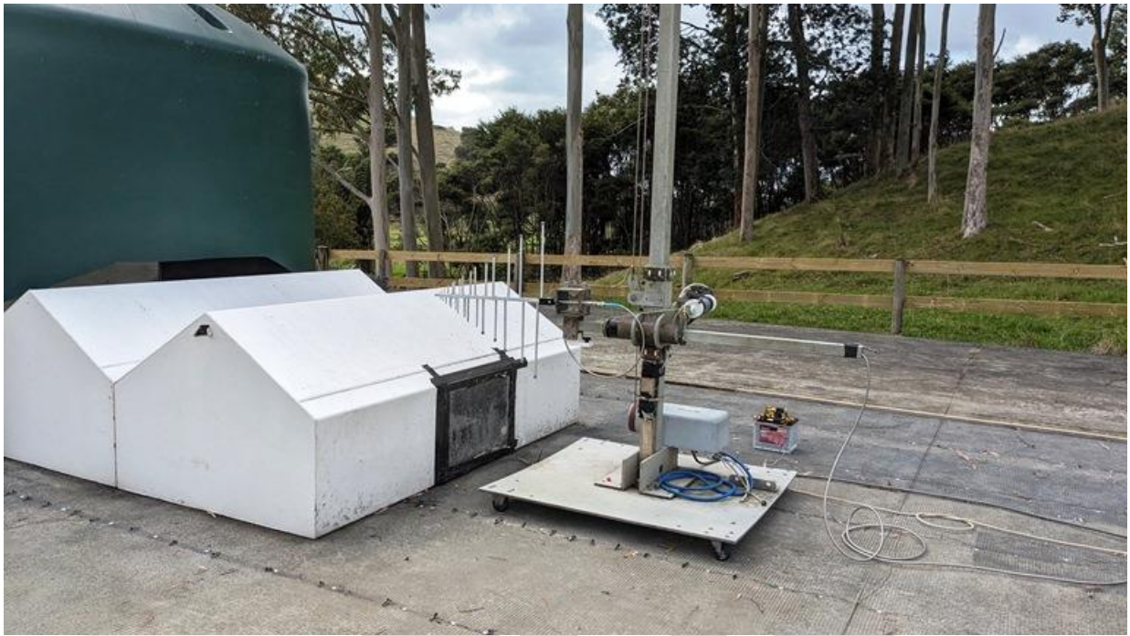
Log Periodic Antenna pointing towards Test Enclosure
