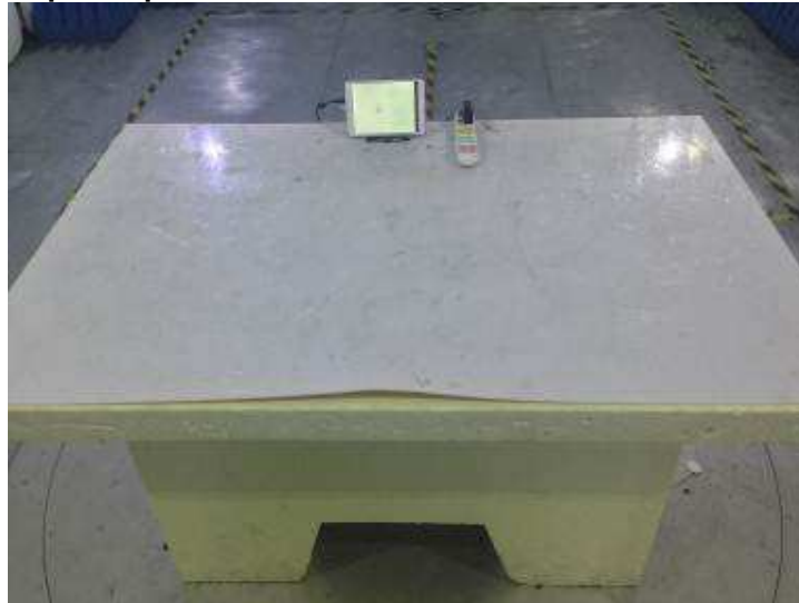
Photograph 2: Set-up for Spurious Emissions
