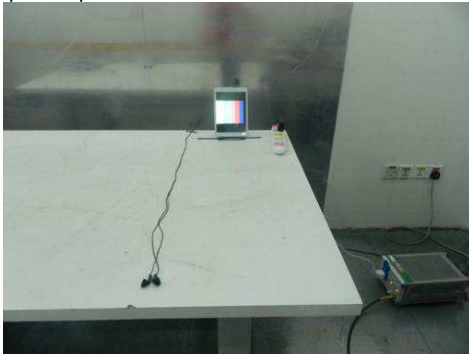
Photograph 1: Set-up for Conducted Emissions
