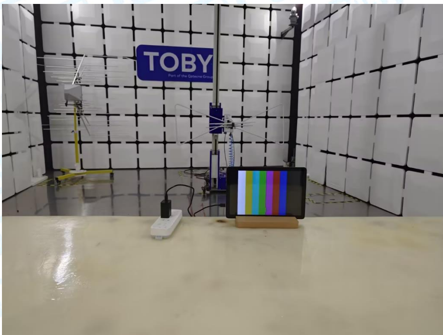
Photo of Setup for Radiated Emission (30MHz~1GHz)
