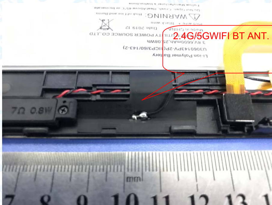
Photo 11 Appearance of Antenna
