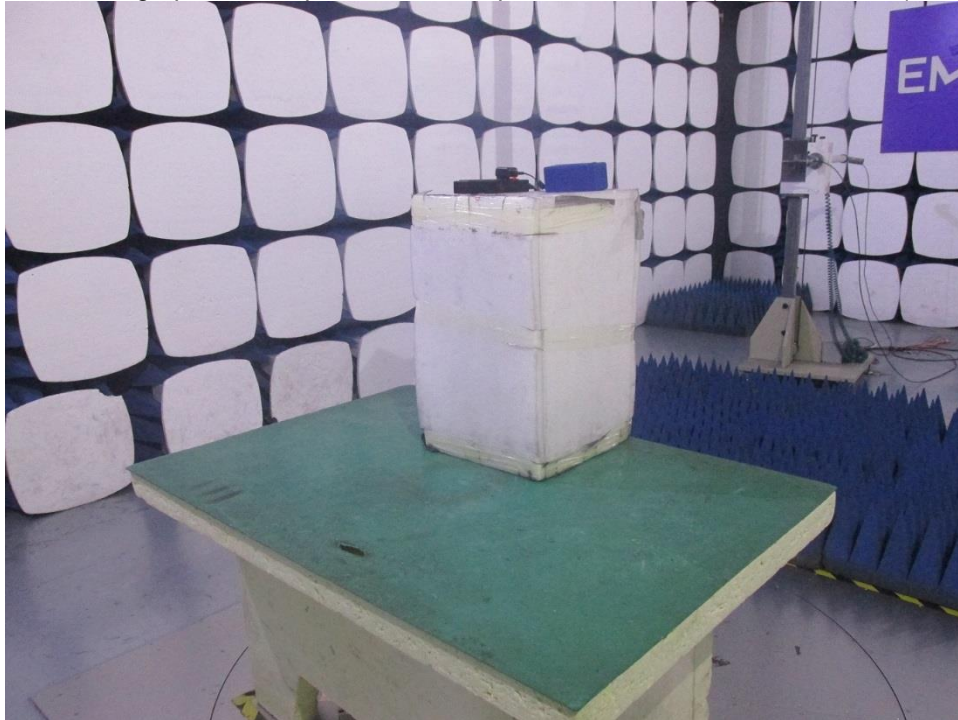
Photograph 4: Set-up for Radiated Spurious Emission above 18GHz
