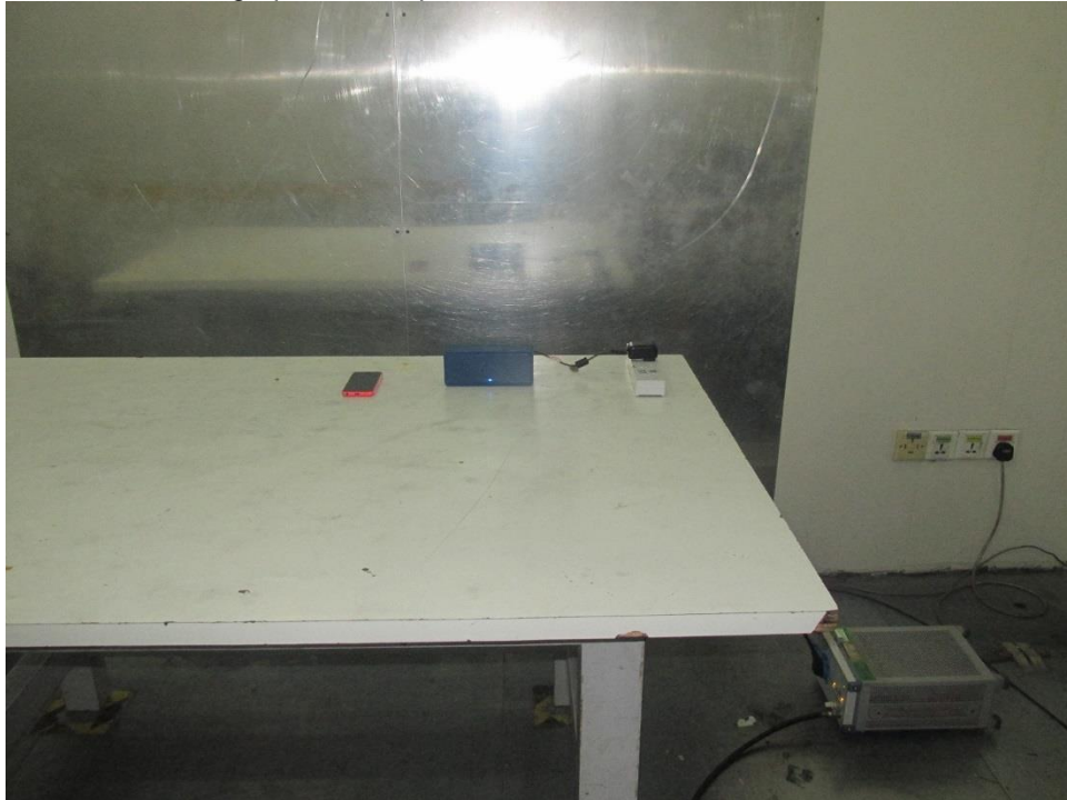
Photograph 5: Set-up for Conducted Emission on AC Mains
