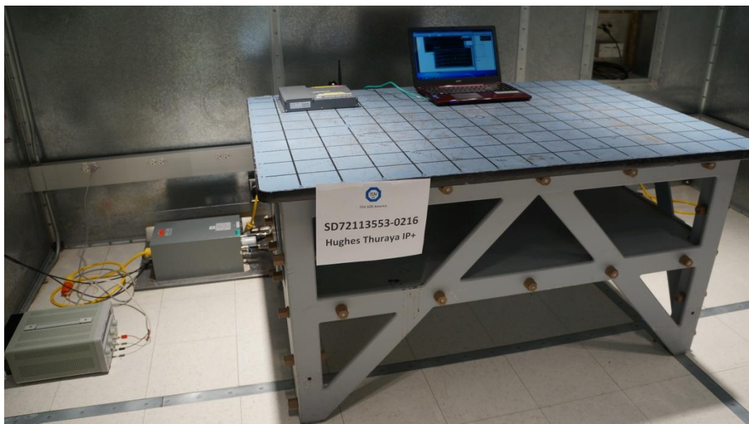
Thuraya 9105, IP Voyager and Orion IP (conducted emission test setup)
