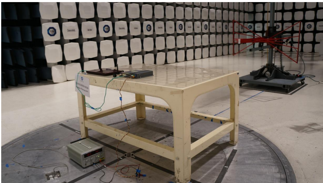
Thuraya 9105, IP Voyager and Orion IP (radiated emission test setup)
