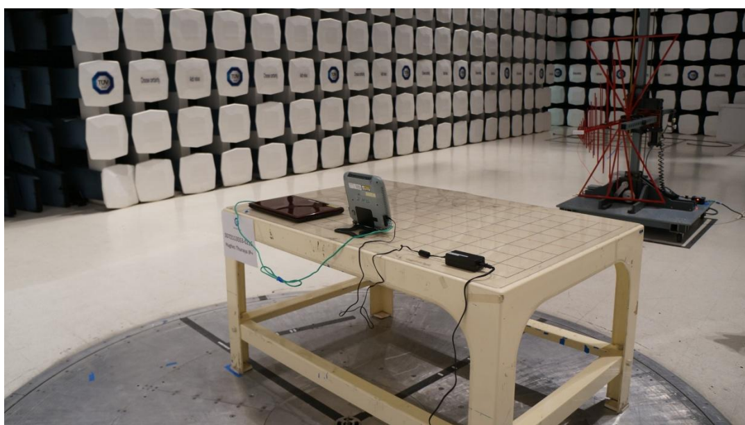
Thuraya 9104, IP+ (radiated emission test setup)
