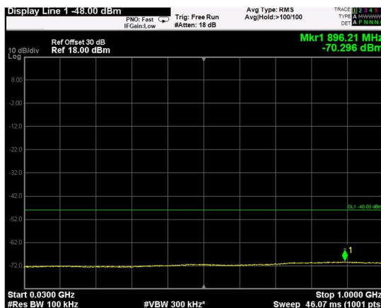
Channel: TOP, Modulation: 64QAM, BW=5MHz, Range: Lower
