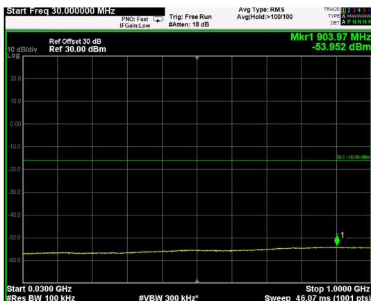
Channel: TOP, Modulation: 256QAM, BW=5MHz, Range: Lower
