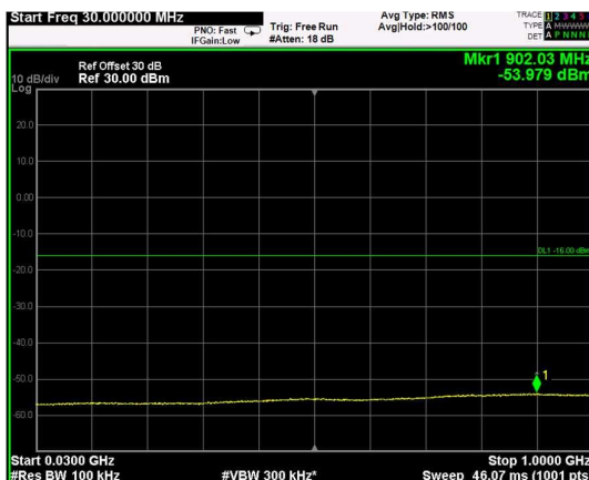
Channel: TOP, Modulation: 64QAM, BW=5MHz, Range: Lower
