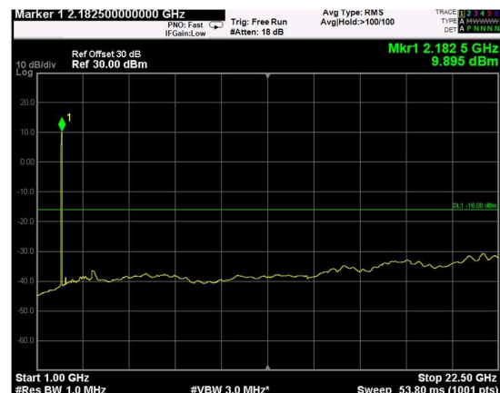
Channel: TOP, Modulation: 256QAM, BW=5MHz, Range: Upper
