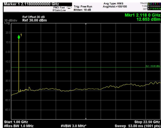
Channel: BOTTOM, Modulation: QPSK, BW=5MHz, Range: Upper
