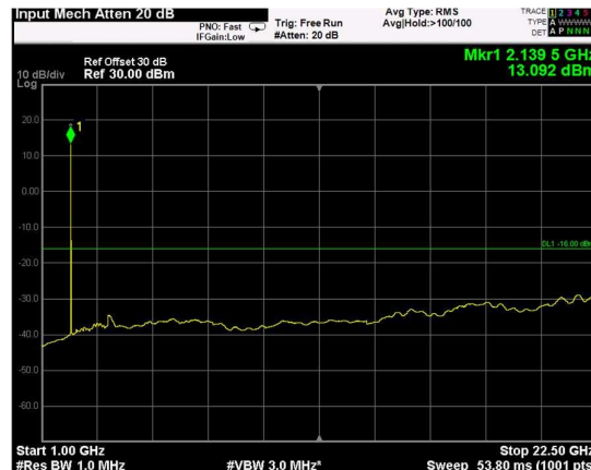
Channel: MIDDLE, Modulation: 256QAM, BW=10MHz, Range: Upper
