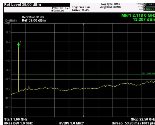
Channel: BOTTOM, Modulation: QPSK, BW=20MHz, Range: Upper
