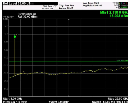
Channel: BOTTOM, Modulation: 256QAM, BW=20MHz, Range: Upper
