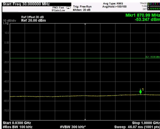
Channel: BOTTOM, Modulation: QPSK, BW=5MHz, Range: Lower
