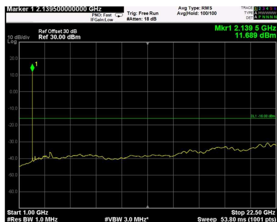
Channel: MIDDLE, Modulation: QPSK, BW=5MHz, Range: Upper
