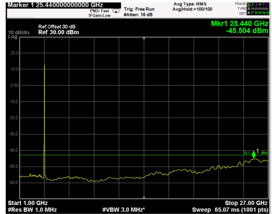
Channel: TOP, Modulation: 256QAM, BW=10MHz, Range: 1GHz - 27GHz
