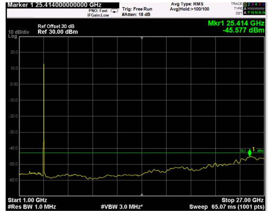
Channel: MIDDLE, Modulation: 256QAM, BW=10MHz, Range: 1GHz - 27GHz
