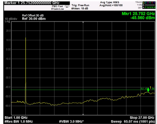
Channel: MIDDLE, Modulation: QPSK, BW=15MHz, Range: 1GHz - 27GHz
