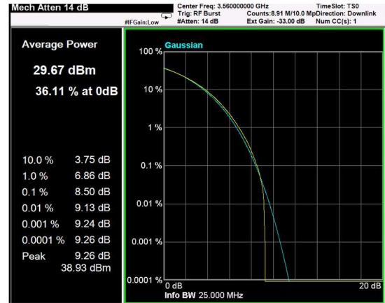
Channel: BOTTOM, Modulation: 256QAM, BW=20MHz, CCDF
