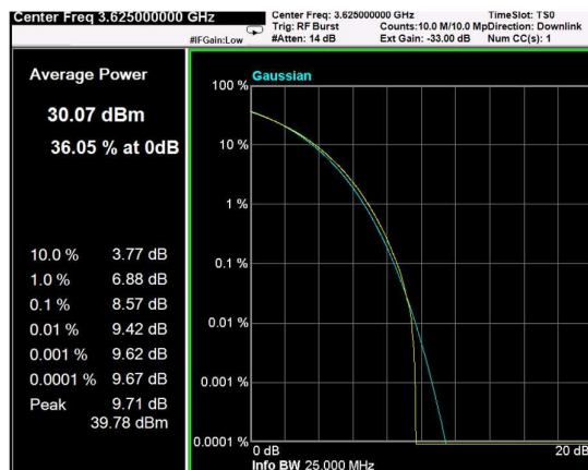
Channel: MIDDLE, Modulation: 64QAM, BW=20MHz, CCDF
