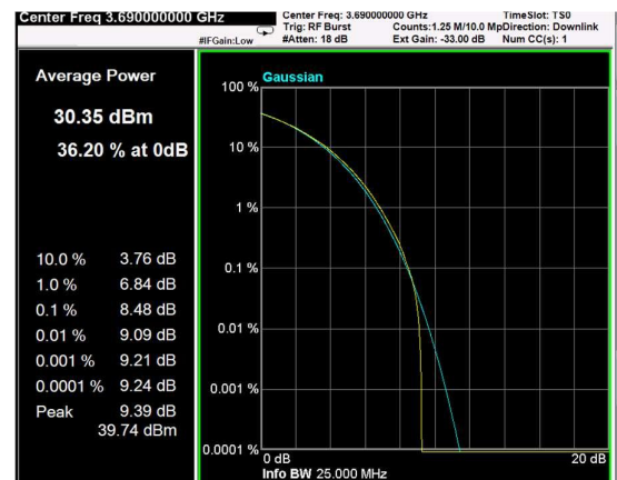
Channel: TOP, Modulation: 256QAM, BW=20MHz, CCDF
