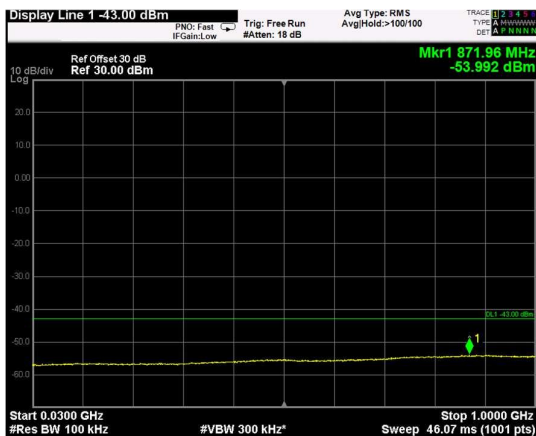
Channel: BOTTOM, Modulation: 16QAM, BW=5MHz, Range: 30MHz - 1GHz
