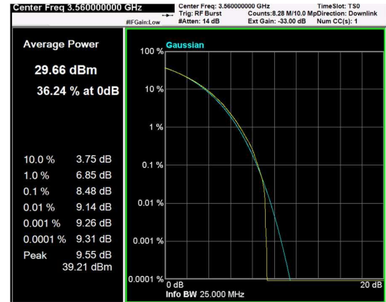
Channel: BOTTOM, Modulation: 64QAM, BW=20MHz, CCDF
