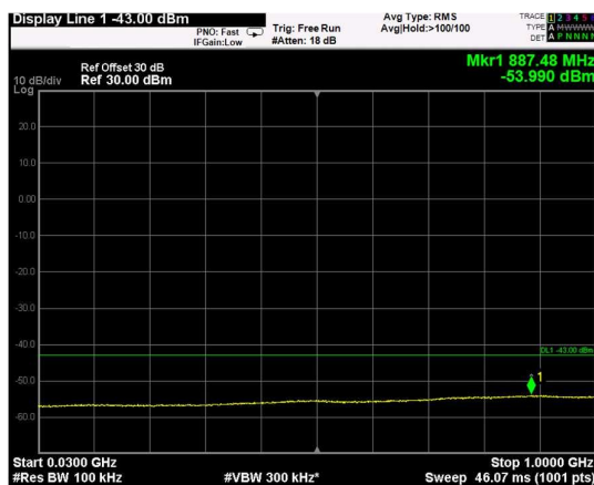
Channel: MIDDLE, Modulation: QPSK, BW=5MHz, Range: 30MHz - 1GHz
