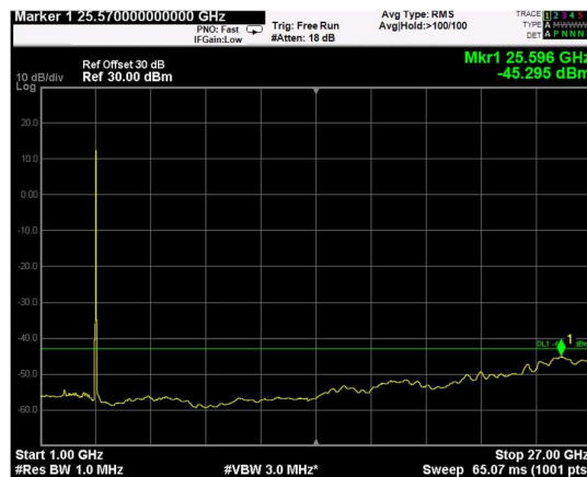
Channel: MIDDLE, Modulation: 16QAM, BW=5MHz, Range: 1GHz - 27GHz
