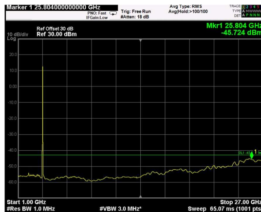
Channel: BOTTOM, Modulation: 16QAM, BW=5MHz, Range: 1GHz - 27GHz
