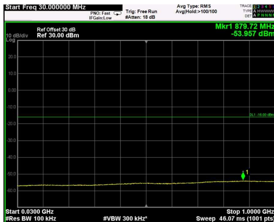
Channel: MIDDLE, Modulation: QPSK, BW=15MHz, Range: Lower
