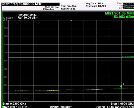
Channel: TOP, Modulation: 64QAM, BW=10MHz, Range: Lower
