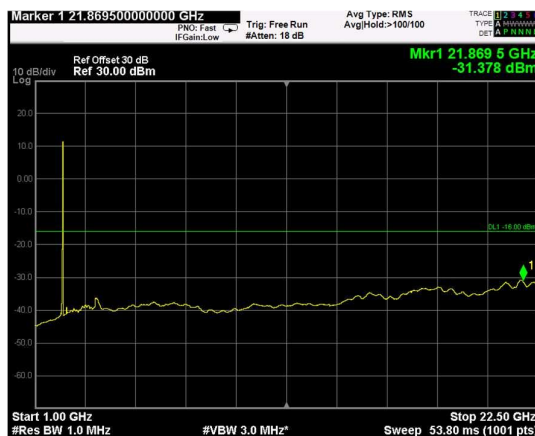
Channel: BOTTOM, Modulation: QPSK, BW=10MHz, Range: Upper
