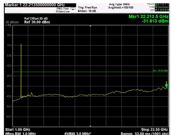
Channel: TOP, Modulation: 256QAM, BW=10MHz, Range: Upper
