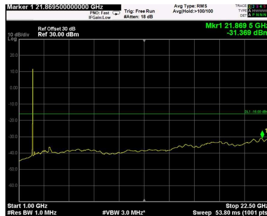
Channel: MIDDLE, Modulation: QPSK, BW=15MHz, Range: Upper
