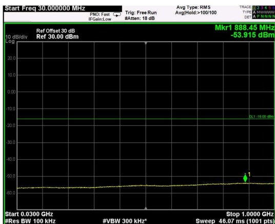
Channel: BOTTOM, Modulation: QPSK, BW=10MHz, Range: Lower
