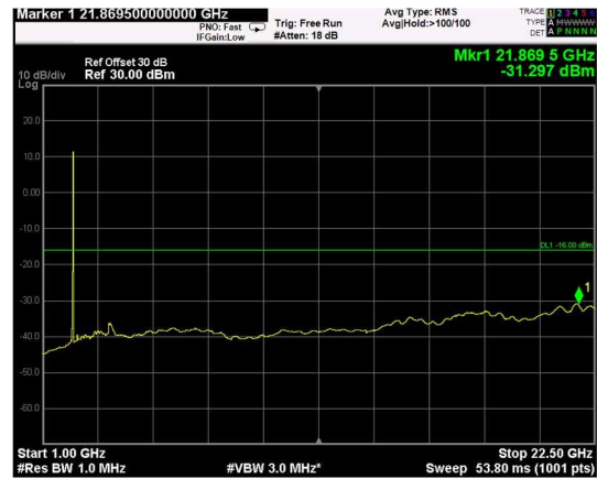
Channel: BOTTOM, Modulation: 64QAM, BW=15MHz, Range: Upper
