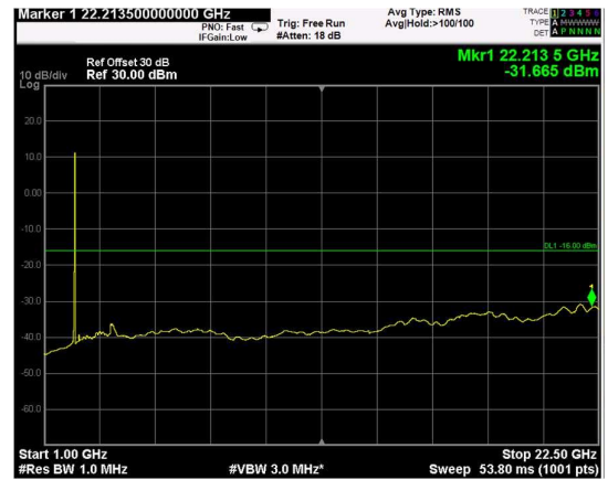
Channel: BOTTOM, Modulation: 256QAM, BW=10MHz, Range: Upper
