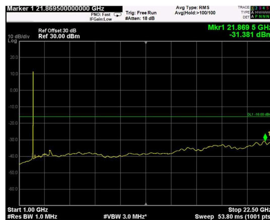
Channel: TOP, Modulation: QPSK, BW=15MHz, Range: Upper
