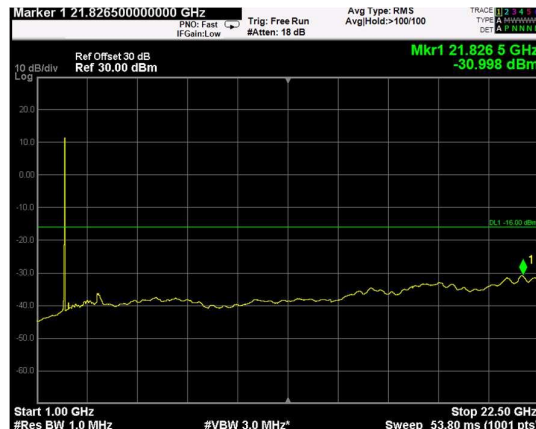
Channel: MIDDLE, Modulation: 64QAM, BW=10MHz, Range: Upper
