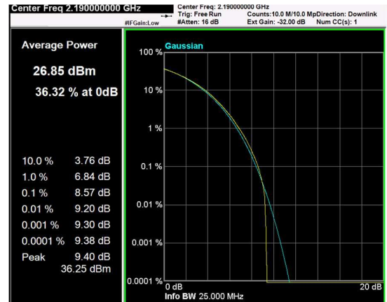
Channel: MIDDLE, Modulation: 16QAM, BW=20MHz, CCDF
