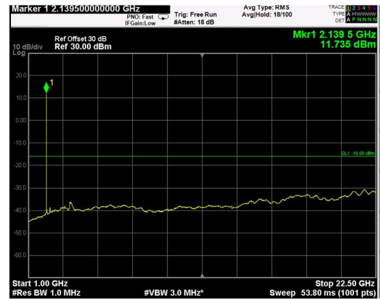
Channel: MIDDLE, Modulation: 16QAM, BW=10MHz, Range: Upper
