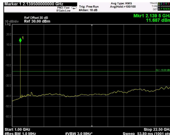
Channel: MIDDLE, Modulation: 256QAM, BW=20MHz, Range: Upper
