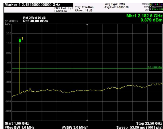
Channel: TOP, Modulation: 16QAM, BW=15MHz, Range: Upper
