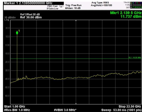
Channel: MIDDLE, Modulation: QPSK, BW=15MHz, Range: Upper
