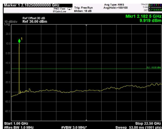
Channel: TOP, Modulation: QPSK, BW=5MHz, Range: Upper
