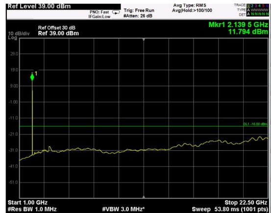
Channel: MIDDLE, Modulation: 64QAM, BW=20MHz, Range: Upper
