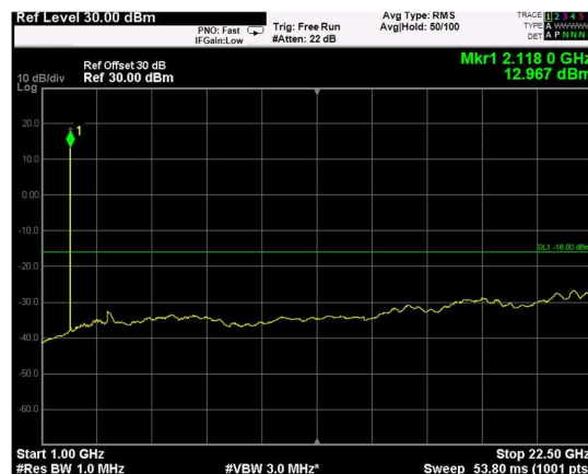
Channel: BOTTOM, Modulation: QPSK, BW=15MHz, Range: Upper
