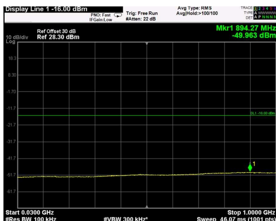
Channel: TOP, Modulation: 256QAM, BW=10MHz, Range: Lower
