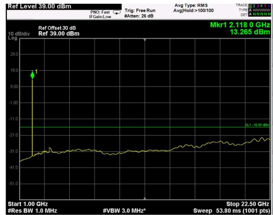
Channel: BOTTOM, Modulation: 64QAM, BW=20MHz, Range: Upper
