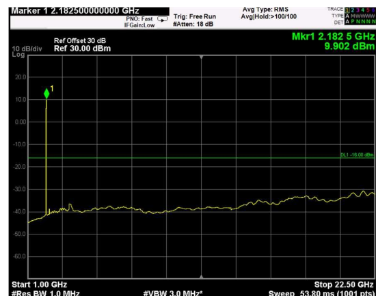
Channel: TOP, Modulation: 64QAM, BW=5MHz, Range: Upper
