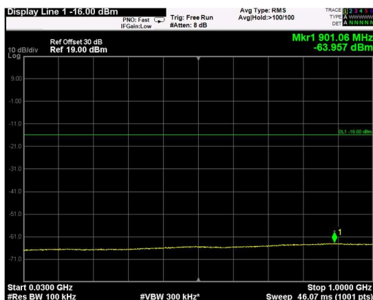
Channel: TOP, Modulation: QPSK, BW=20MHz, Range: Lower
