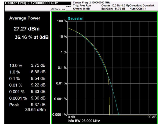
Channel: BOTTOM, Modulation: 64QAM, BW=20MHz, CCDF
