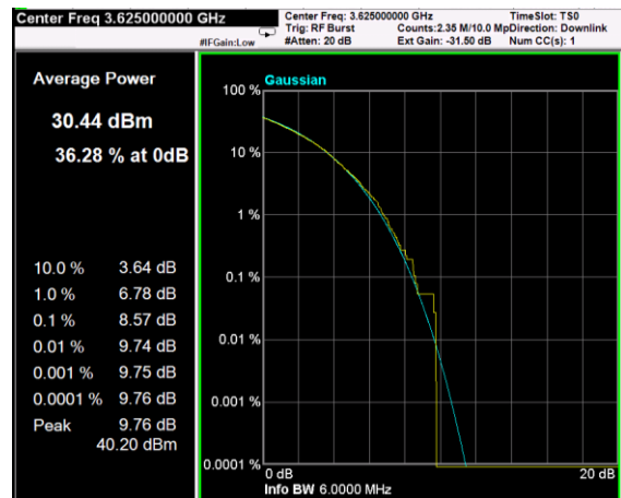
Channel: MIDDLE, Modulation: 256QAM, BW=5MHz, CCDF
