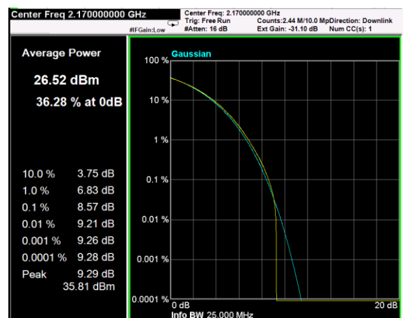
Channel: TOP, Modulation: 16QAM, BW=20MHz, CCDF
