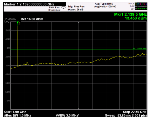
Channel: MIDDLE, Modulation: 256QAM, BW=15MHz, Range: Upper
