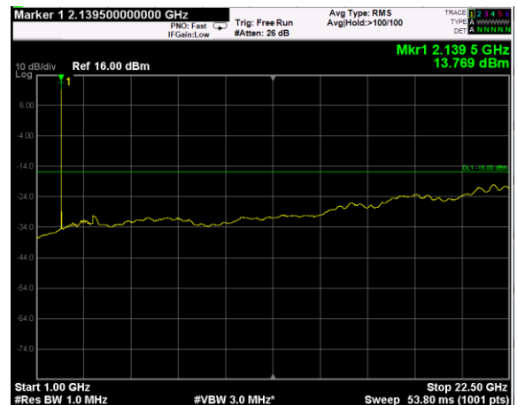
Channel: MIDDLE, Modulation: 16QAM, BW=5MHz, Range: Upper
