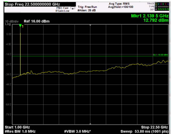
Channel: MIDDLE, Modulation: QPSK, BW=20MHz, Range: Upper
