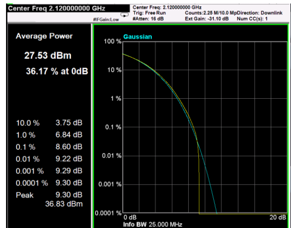
Channel: BOTTOM, Modulation: QPSK, BW=20MHz, CCDF
