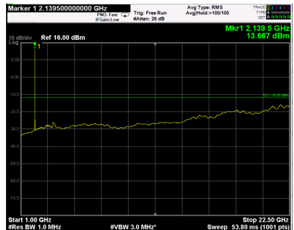
Channel: MIDDLE, Modulation: 64QAM, BW=5MHz, Range: Upper
