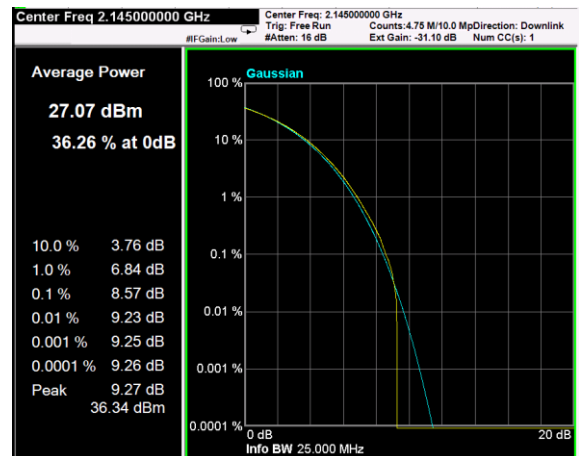
Channel: MIDDLE, Modulation: 16QAM, BW=20MHz, CCDF
