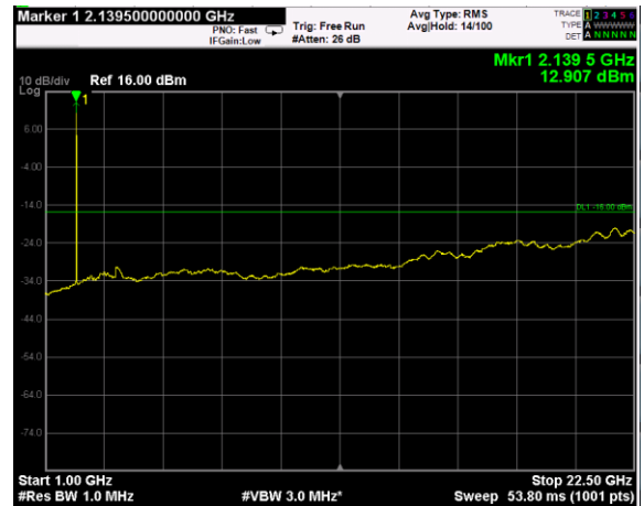
Channel: MIDDLE, Modulation: QPSK, BW=15MHz, Range: Upper
