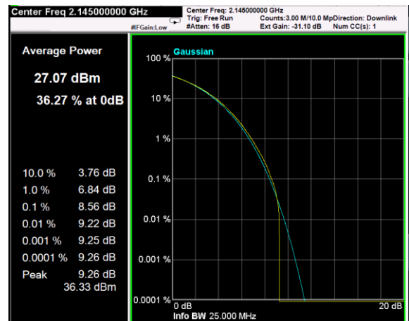
Channel: MIDDLE, Modulation: 256QAM, BW=20MHz, CCDF
