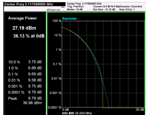
Channel: BOTTOM, Modulation: 256QAM, BW=15MHz, CCDF
