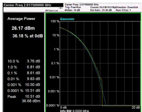
Channel: TOP, Modulation: 64QAM, BW=5MHz, CCDF
