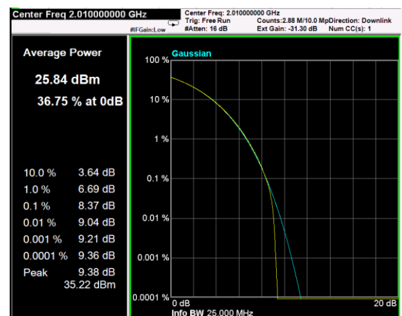
Channel: TOP, Modulation: 16QAM, BW=20MHz, CCDF
