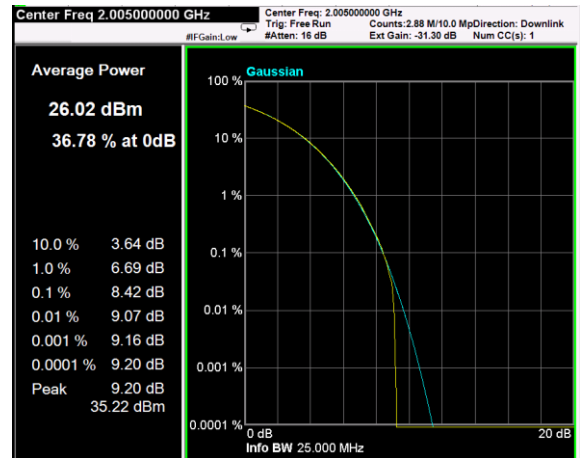
Channel: BOTTOM, Modulation: QPSK, BW=20MHz, CCDF
