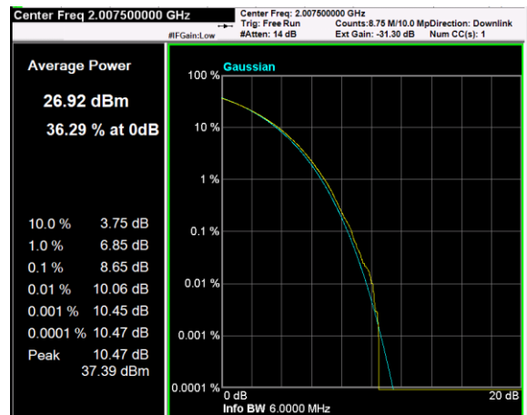
Channel: MIDDLE, Modulation: 64QAM, BW=5MHz, CCDF
