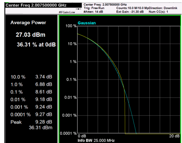
Channel: MIDDLE, Modulation: QPSK, BW=10MHz, CCDF
