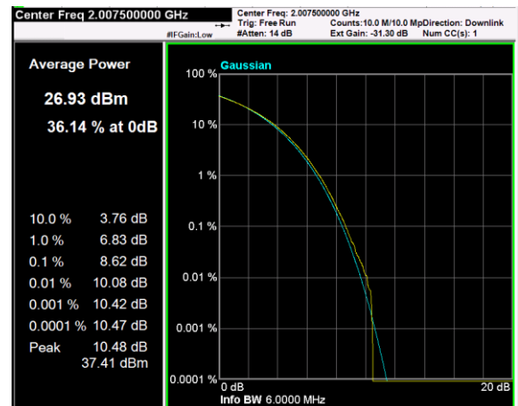
Channel: MIDDLE, Modulation: 16QAM, BW=5MHz, CCDF
