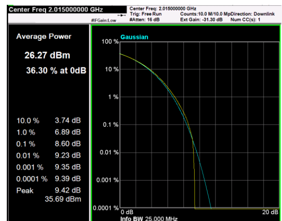
Channel: TOP, Modulation: QPSK, BW=10MHz, CCDF
