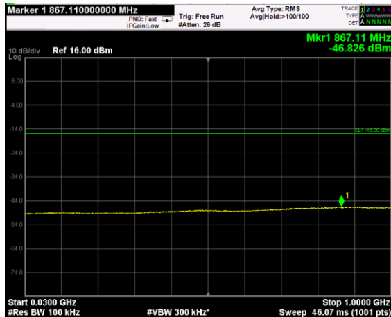
Channel: MIDDLE, Modulation: QPSK, BW=20MHz, Range: Lower
