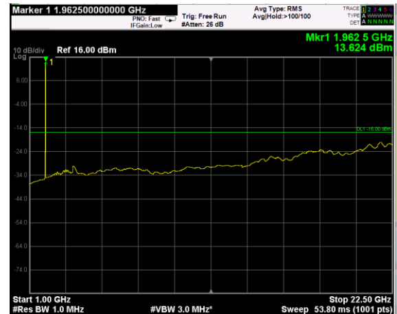
Channel: MIDDLE, Modulation: QPSK, BW=15MHz, Range: Upper
