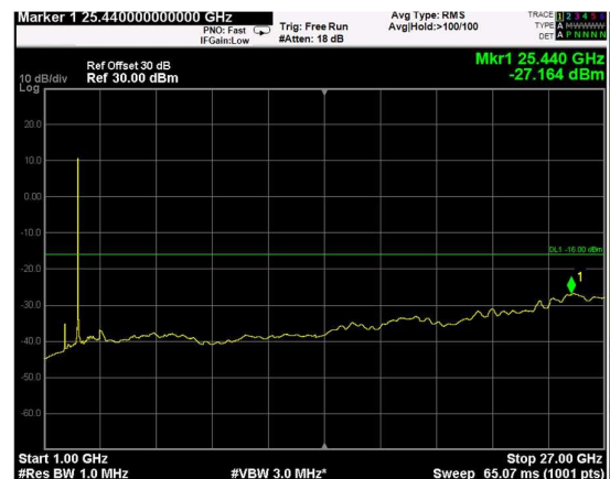
Channel: TOP, Modulation: 64QAM, BW=10MHz, Range: Upper
