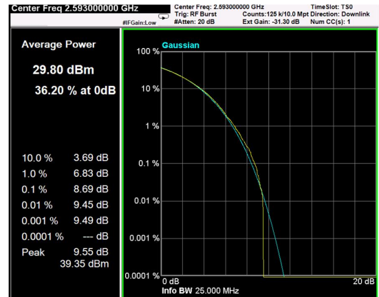
Channel: MIDDLE, Modulation: QPSK, BW=15MHz, CCDF
