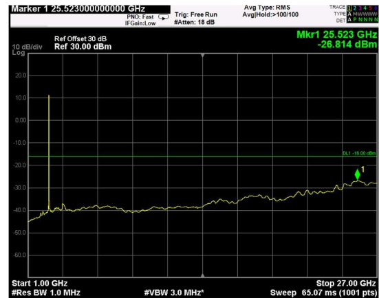
Channel: MIDDLE, Modulation: 16QAM, BW=5MHz, Range: Upper
