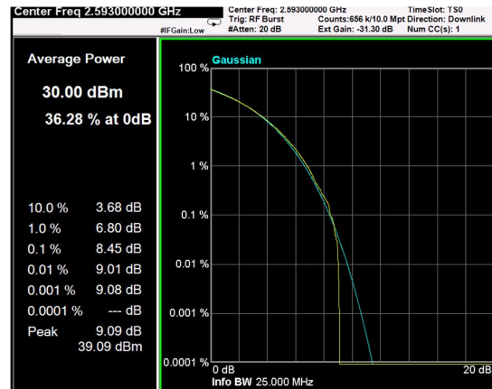
Channel: MIDDLE, Modulation: 256QAM, BW=20MHz, CCDF
