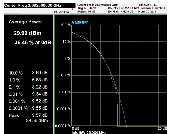
Channel: TOP, Modulation: QPSK, BW=15MHz, CCDF
