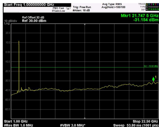
Channel: BOTTOM, Modulation: QPSK, BW=10MHz, Range: Upper
