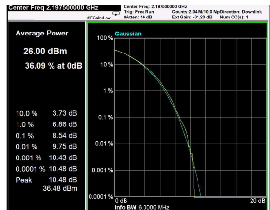
Channel: TOP, Modulation: 64QAM, BW=5MHz, CCDF
