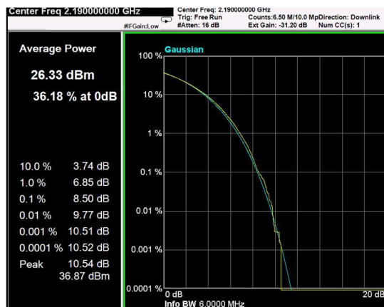
Channel: MIDDLE, Modulation: 16QAM, BW=5MHz, CCDF
