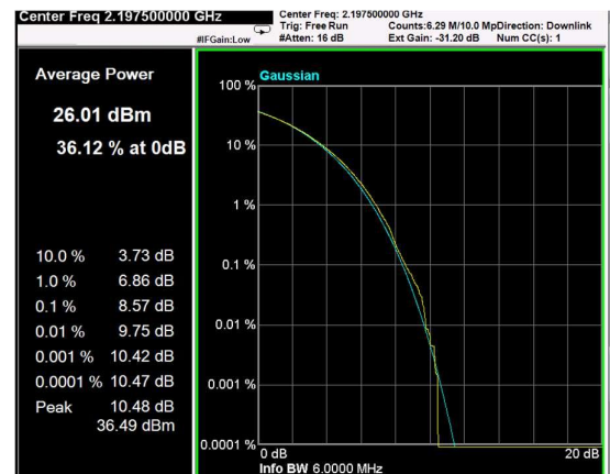
Channel: TOP, Modulation: QPSK, BW=5MHz, CCDF
