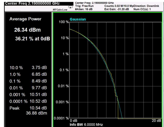
Channel: MIDDLE, Modulation: 64QAM, BW=5MHz, CCDF
