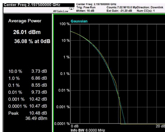
Channel: TOP, Modulation: 16QAM, BW=5MHz, CCDF
