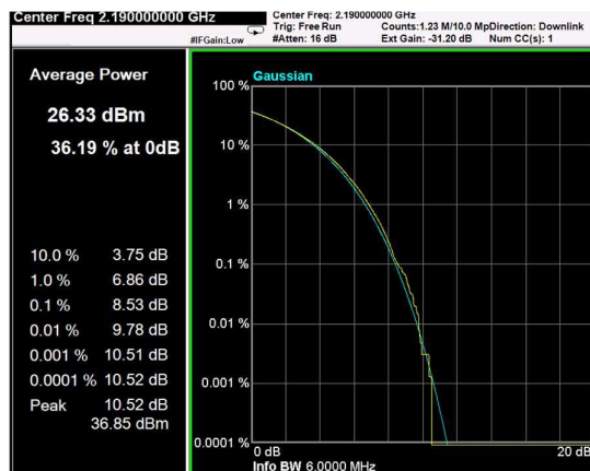
Channel: MIDDLE, Modulation: 256QAM, BW=5MHz, CCDF
