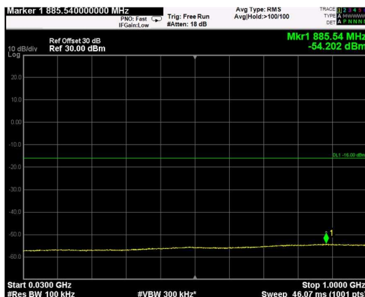
Channel: TOP, Modulation: 64QAM, BW=15MHz, Range: Lower
