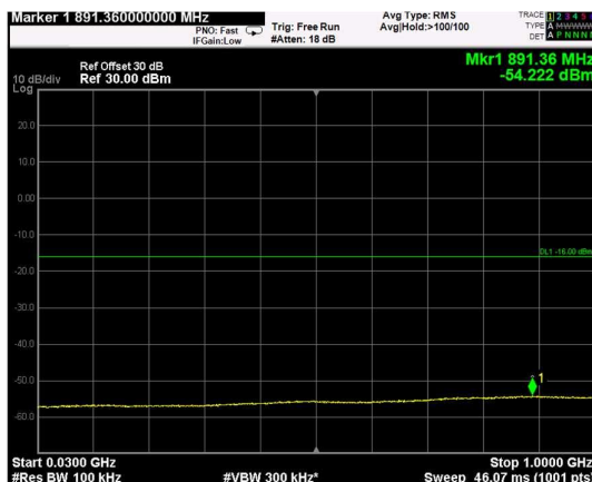
Channel: TOP, Modulation: 256QAM, BW=20MHz, Range: Lower
