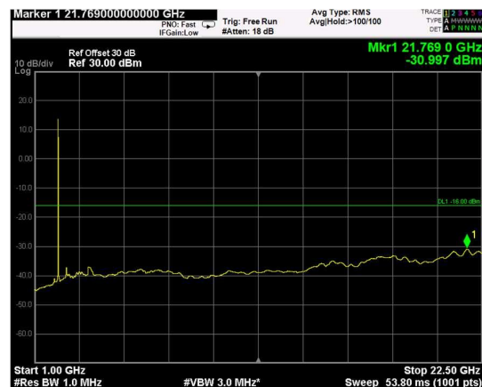
Channel: TOP, Modulation: 16QAM, BW=15MHz, Range: Upper
