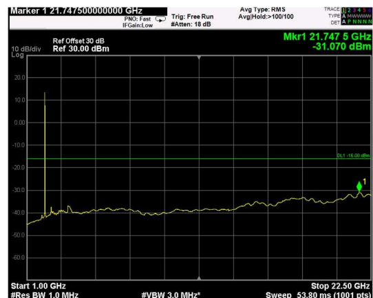
Channel: TOP, Modulation: 64QAM, BW=15MHz, Range: Upper
