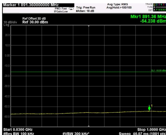
Channel: TOP, Modulation: 256QAM, BW=20MHz, Range: Lower
