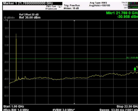
Channel: MIDDLE, Modulation: 16QAM, BW=20MHz, Range: Upper
