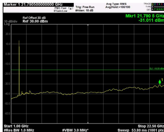
Channel: BOTTOM, Modulation: 16QAM, BW=20MHz, Range: Upper
