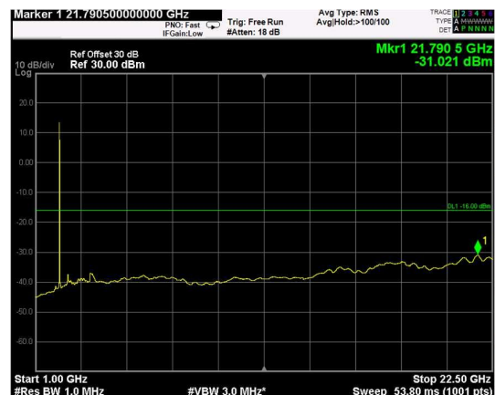
Channel: TOP, Modulation: 64QAM, BW=20MHz, Range: Upper
