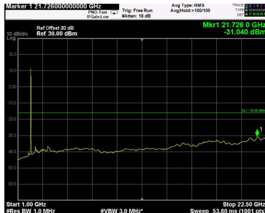
Channel: MIDDLE, Modulation: 256QAM, BW=5MHz, Range: Upper
