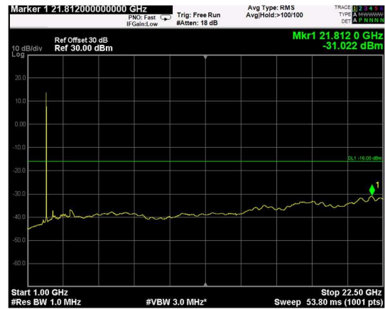
Channel: BOTTOM, Modulation: 256QAM, BW=15MHz, Range: Upper
