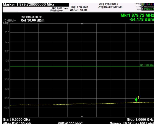
Channel: TOP, Modulation: 256QAM, BW=5MHz, Range: Lower
