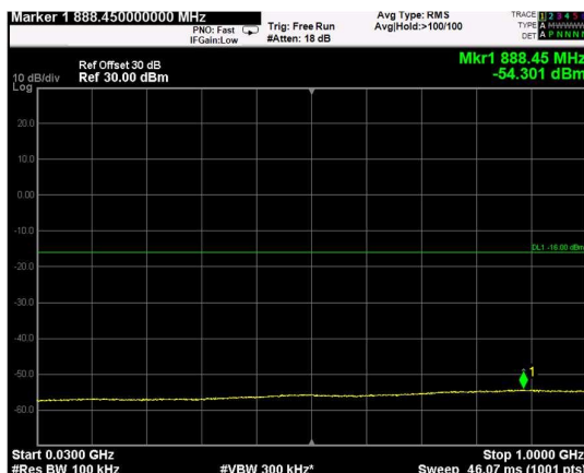
Channel: TOP, Modulation: 16QAM, BW=20MHz, Range: Lower
